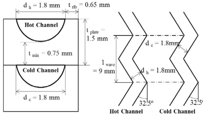
**Figure 5. Channel geometry of designed S-CO<sub>2</sub> to water heat exchanger**
