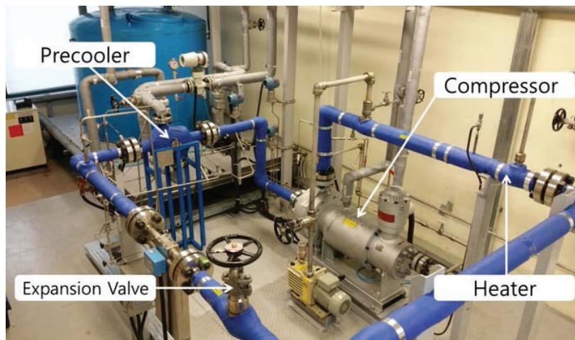
**Figure 7. Overall view of the S-CO<sub>2</sub>PE facility**
