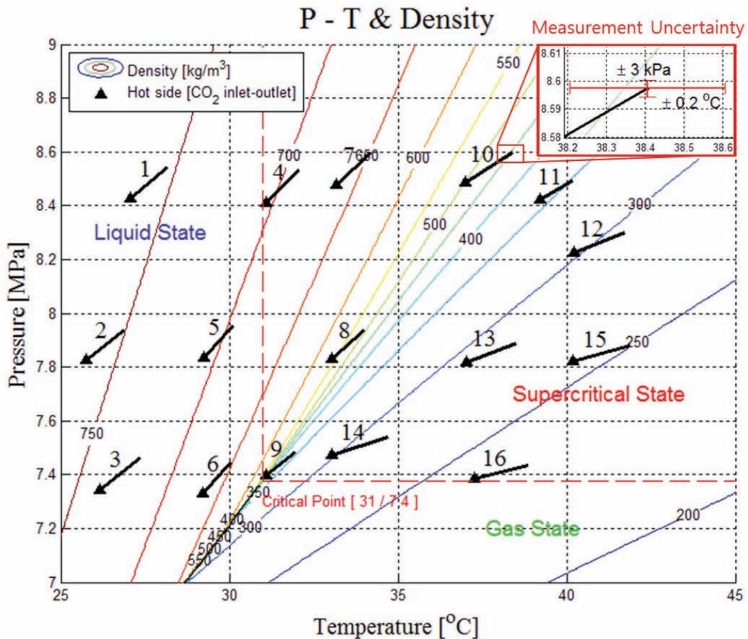
Figure 8. S-CO<sub>2</sub> inlet-outlet condition of tested cases
