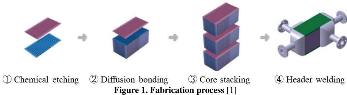
**Figure 1. Fabrication process [1]**
