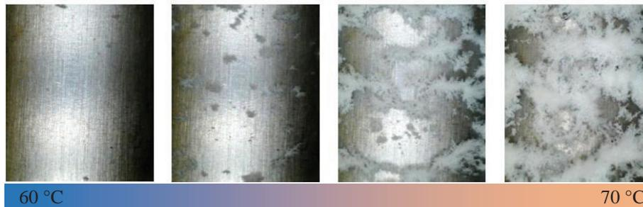
**Figure 10. Development of a deposit layer on heating rod surface for local fluid temperature range of 60-70 °C (exp.no. RLII-HZ9-V08, starting concentrations: Zn 86.2 mg/L; boric acid: 13 g/L)**
