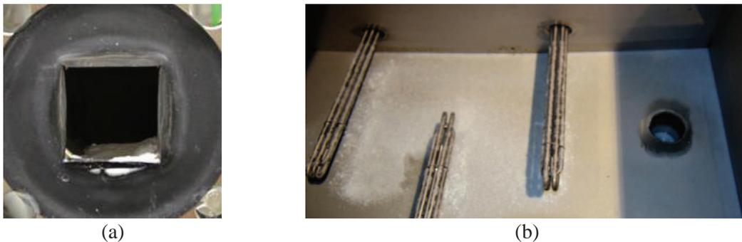
**Figure 9. Sediments of zinc corrosion products at the outlet of the HC (a) and in the water reservoir (b) in experiment no. RLII-HZ9-V20**
