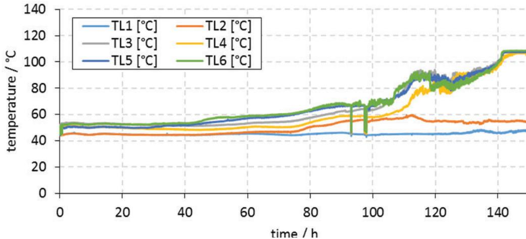
Figure 13. Coolant temperatures between the heated rods during the first 6 days of the experiment no. ZFT-BE-V08 (TL1-TL6: from outside to the inside of the FA dummy)
