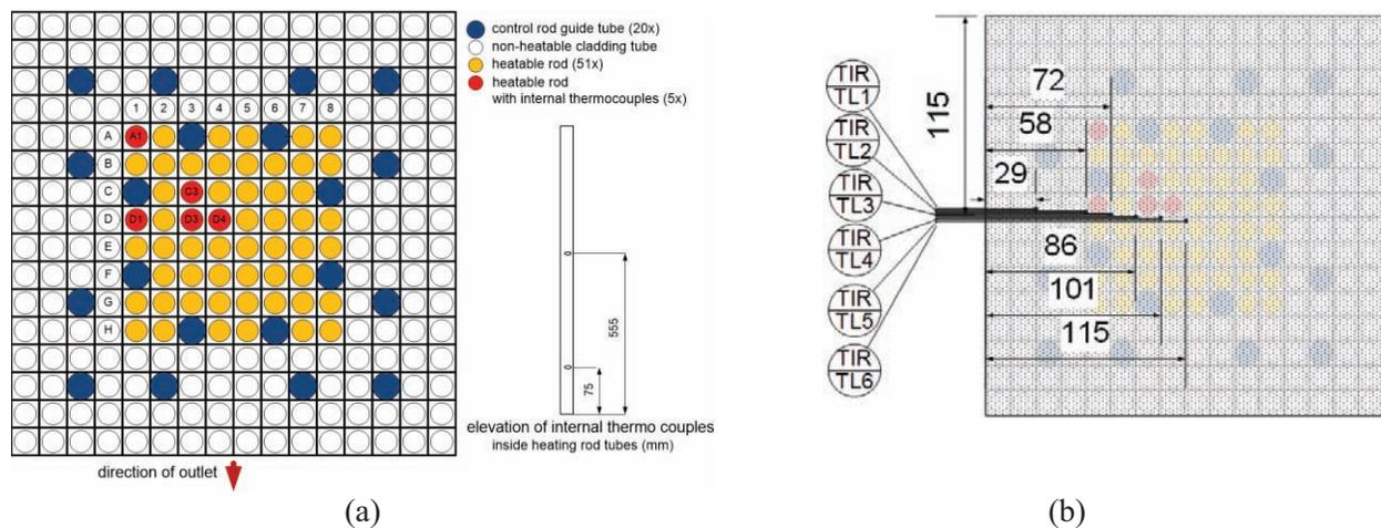
Figure 5. Position scheme of the heating rods, in part equipped with TC (a), TC placed in coolant between the tubes (b)
