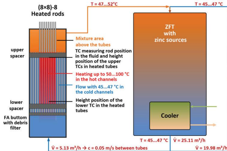
Figure 4. Scheme of the ZFT with partially heatable FA dummy
