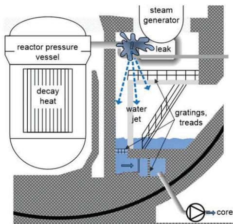
Figure 1. Scheme of a LOCA scenario inside a PWR
