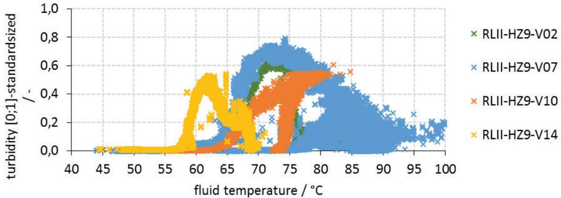
Figure 7. Turbidity and local fluid temperature at the HC outlet for selected experiments
