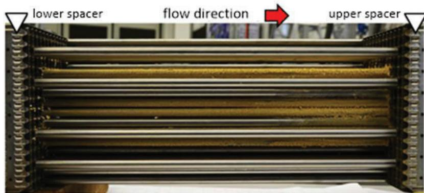
**Figure 15. Layers of zinc corrosion products on heating rod surfaces of the FA dummy after experiment no. ZSW-BE-V02 (boric acid: 13g/l; Li: 0.5 ppm)**
