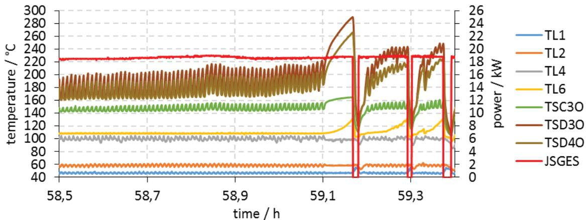
Figure 14. Oscillating coolant temperatures (TLx)/internal rod temperatures (TSxx) and total heat output (JSGES) in experiment no. ZFT-BE-V02
