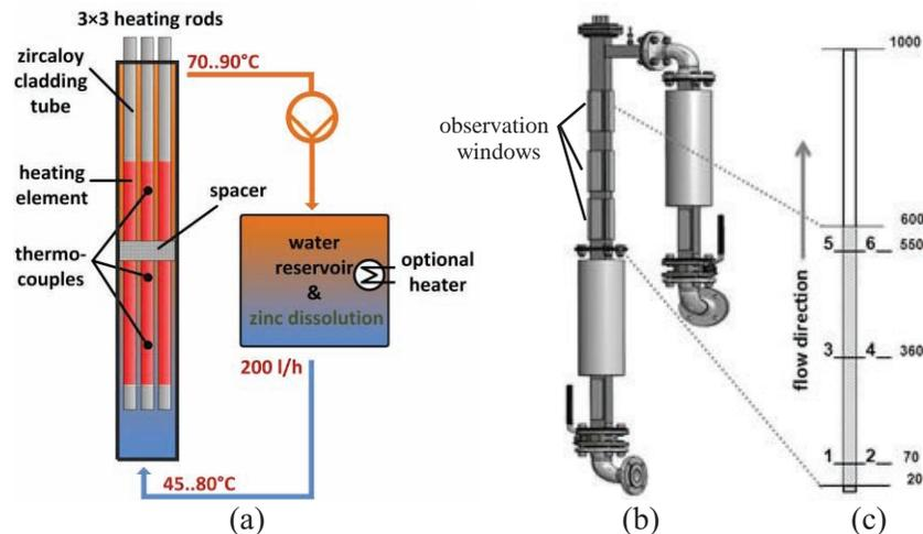
**Figure 2. Scheme of the test facility "Ring line II" (a), equipped with an observation part (b) and a 3×3 configuration of heating rods with integrated thermocouples (c)**
