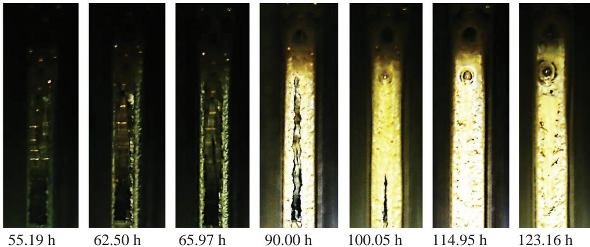
Figure 12. Development of a solid deposit layer between the heating rods upstream of the spacer (experiment no. ZFT-BE-V03)
