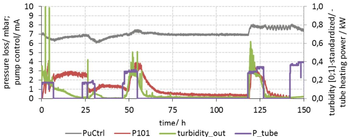
Figure 8. Pump control current, turbidity, head loss and heating power in experiment no. RLII-HZ9-V20
