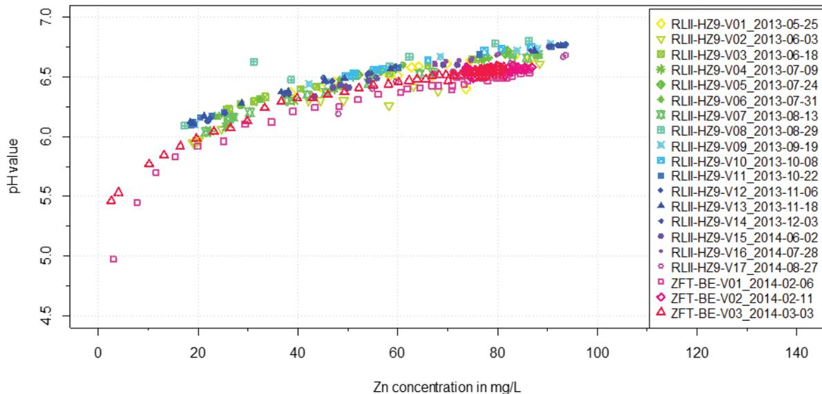
Figure 17. Zn concentration in coolant vs. pH (Test rig RLII and ZFT)
