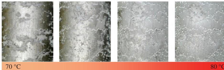
**Figure 11. Development of a deposit layer on heating rod surface for local fluid temperature range of 70-80 °C (exp.no. RLII-HZ9-V08, starting concentrations: Zn 86.2 mg/l; boric acid: 13 g/l)**
