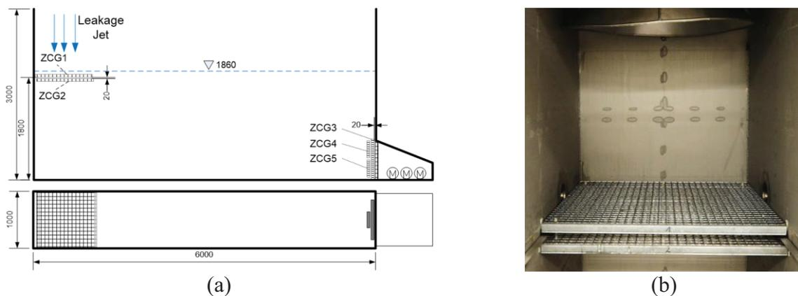
Figure 3. Positions of the ZCG in the ZFT in side and top view (a), ZCG mounted below leaking jet position in the ZFT (b)
