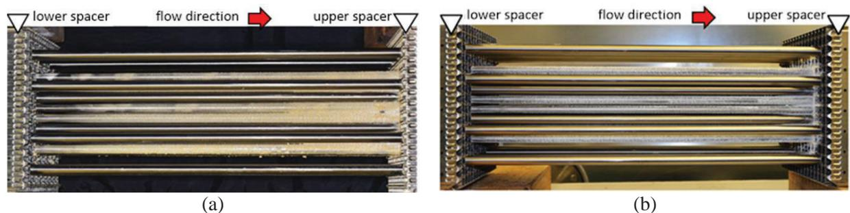
**Figure 16. Layers of zinc corrosion products on heating rod surfaces of the FA dummy after the experiment with 15 ppm (a) and 38 ppm lithium (b)**
