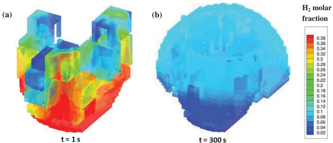
Figure 4. 3D visualization of hydrogen distribution: (a) initial jet; (b) stratified cloud.
