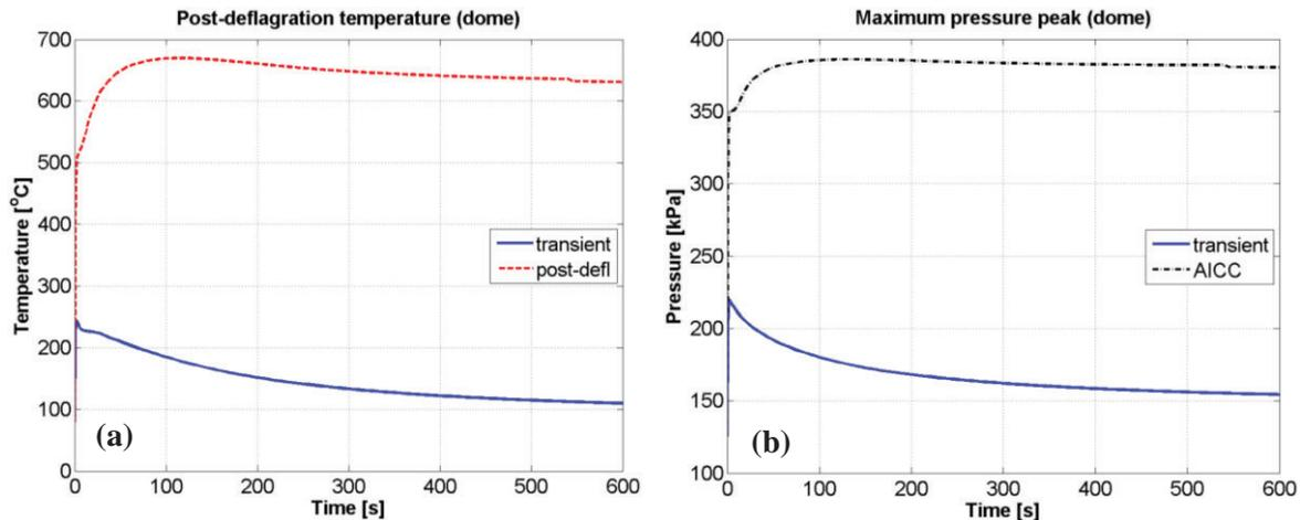
**Figure 11. Computation of post-deflagration temperature (a) and AICC pressure value (b) for average conditions in containment dome (Vol.1s). Base case results.**
