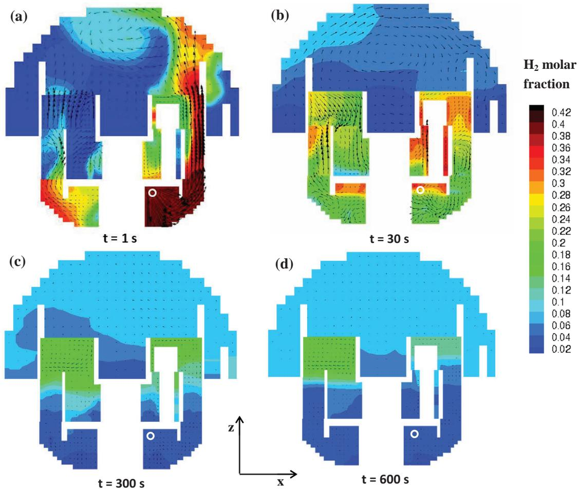
Figure 6. Contour maps of hydrogen concentration: steam generator dampers closing case.
