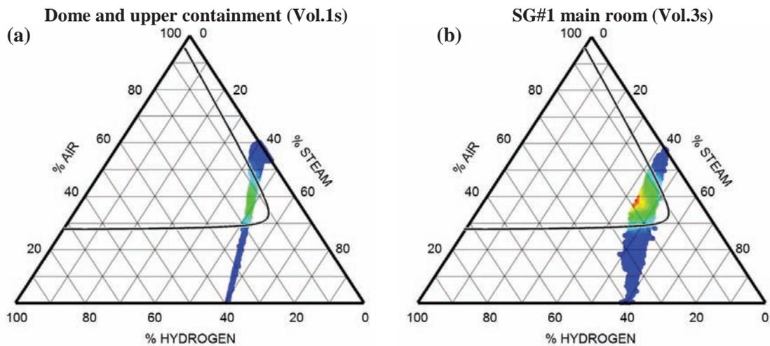
Figure 10. Trajectory clouds on the Shapiro diagram (1000 s transient): sensitivity with dampers closing.
