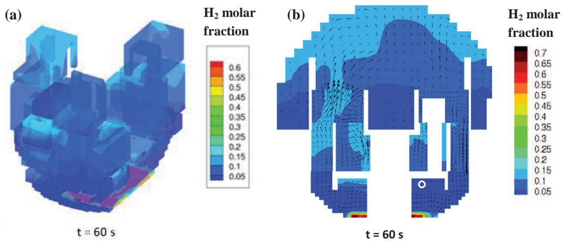
Figure 7. High local hydrogen concentration computed in the sump zone: (a) 3D view; (b) 2D contour map.
