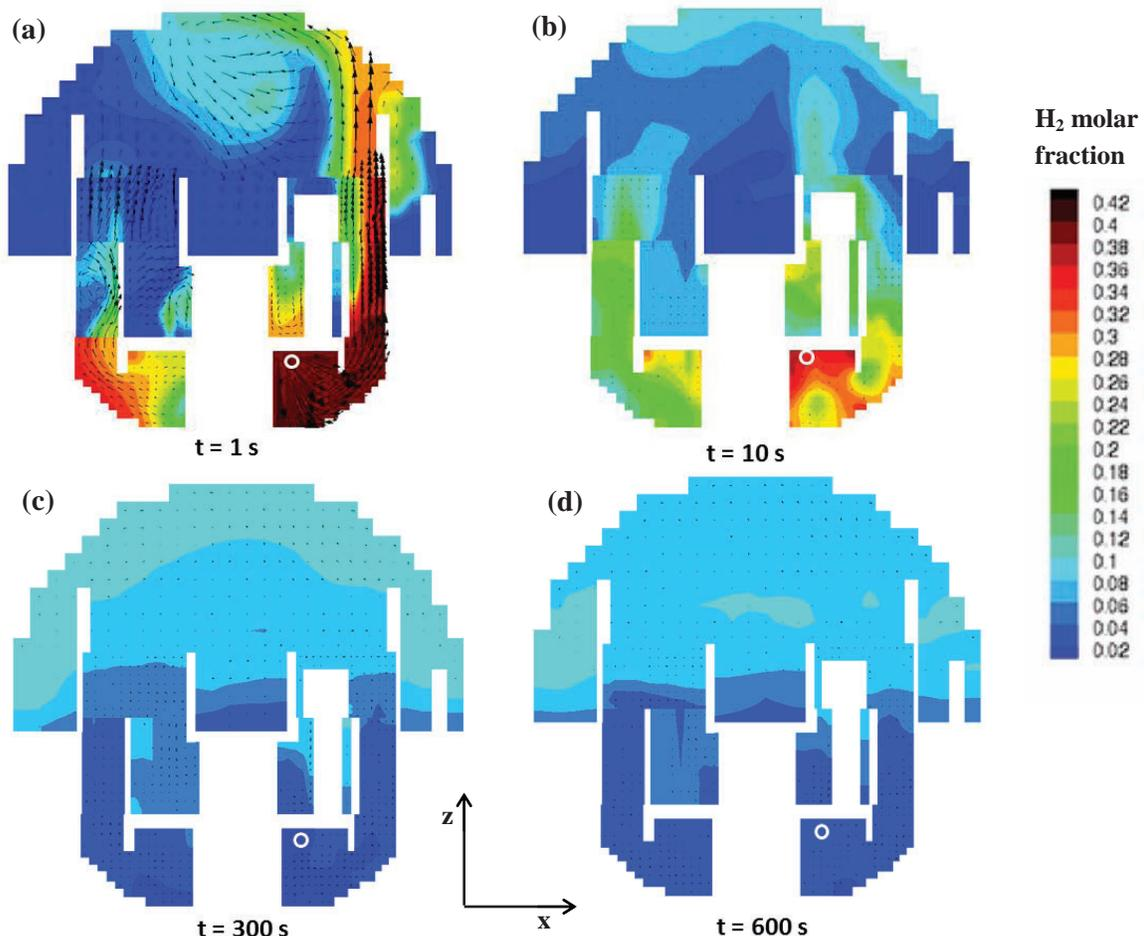
Figure 3. Contour maps of hydrogen concentration: base case transient sequence.
