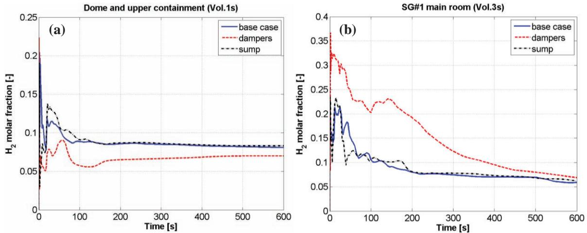
**Figure 8. Comparison of hydrogen concentration in selected cells (top location) in upper containment volume (a) and steam generator compartment (b).**
