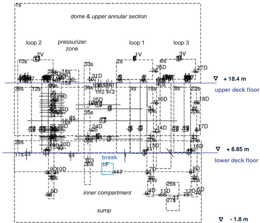
Figure 1. GOTHIC nodalization diagram of the containment.
