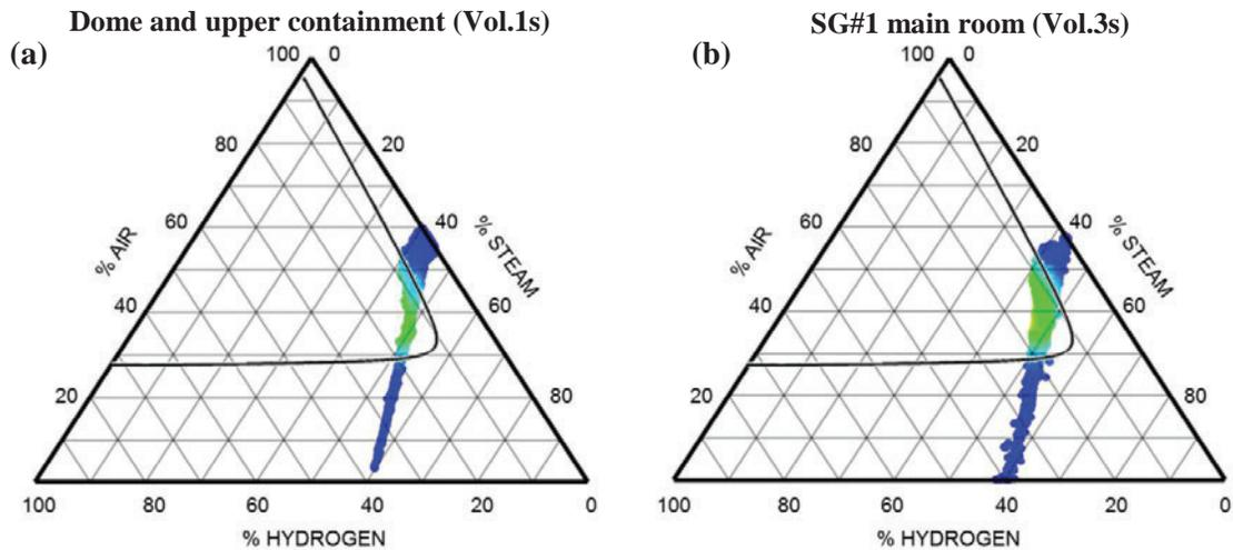
Figure 9. Trajectory clouds on the Shapiro diagram (1000 s transient): base case.
