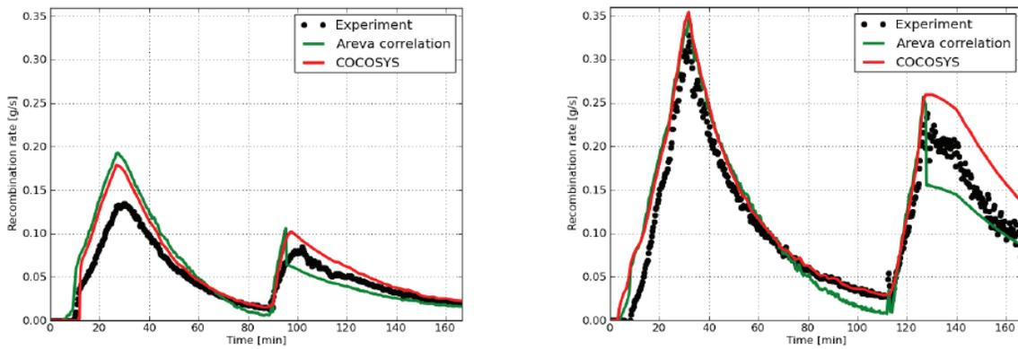
Figure 5. Comparison of measured and calculated  $H_2$  recombination rate, experiments with 60 % steam: THAI HR-13 1.0 bar (left), THAI HR-12 3.0 bar (right) [13].
