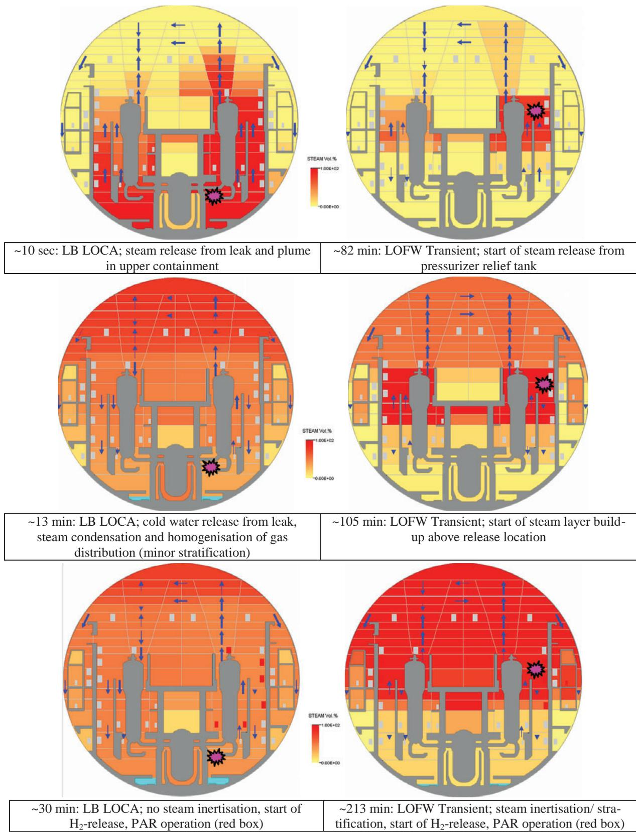
**Figure 8. Steam concentration in PWR containment prior to H<sub>2</sub> release.**
