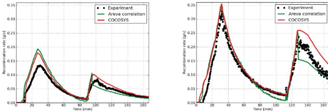
Figure 5. Comparison of measured and calculated H<sub>2</sub> recombination rate, experiments with 60 % steam: THAI HR-13 1.0 bar (left), THAI HR-12 3.0 bar (right) [13].
