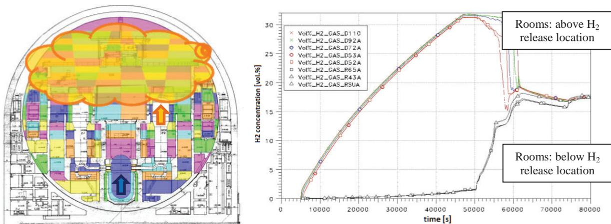
**Figure 7. Test of PWR nodalisation to reproduce build-up of H<sub>2</sub> stratification above release location and dissolution by steam release from cavity; right: H<sub>2</sub> concentration in different rooms [10].**
