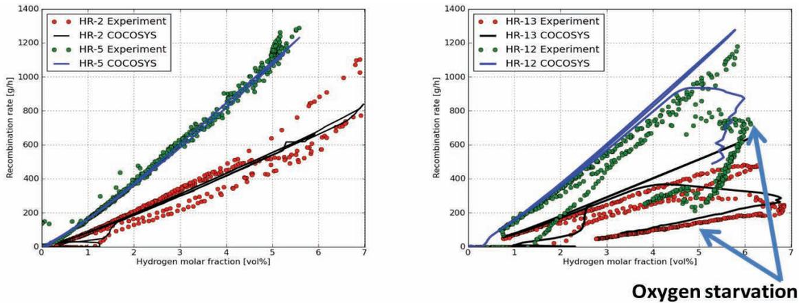
Figure 6. Comparison of measured and calculated  $H_2$  recombination rate versus  $H_2$  molar fraction in different THAI HR experiments, without steam (left) and with saturated conditions (right) [13].
