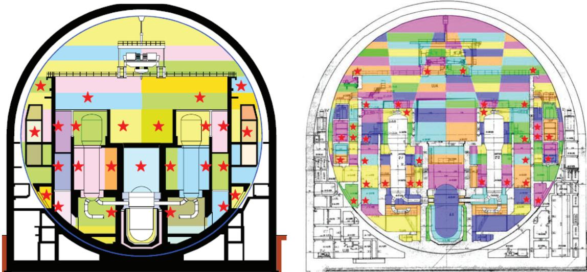
Figure 2. COCOSYS nodalisation schemes with PAR location (red stars); left: “basic PAR concept” and scheme used first [9], right: “realized PAR concept” and scheme used for re-evaluation [10].
