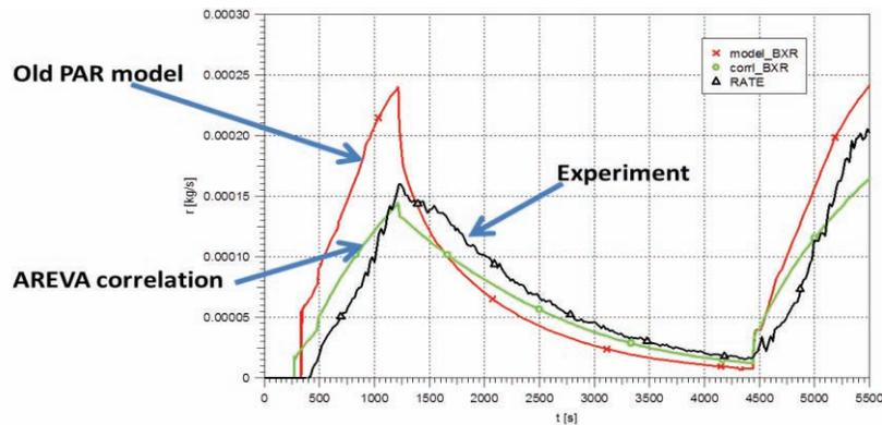
Figure 3. H<sub>2</sub> recombination rate, no steam: THAI HR-5 3.3 bar [13].
