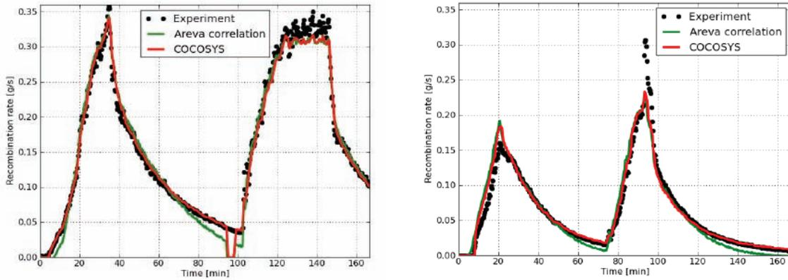
Figure 4. Comparison of measured and calculated  $H_2$  recombination rate, experiments without steam: THAI HR-2 1.0 bar (left); THAI HR-5 3.3 bar (right) [13].
