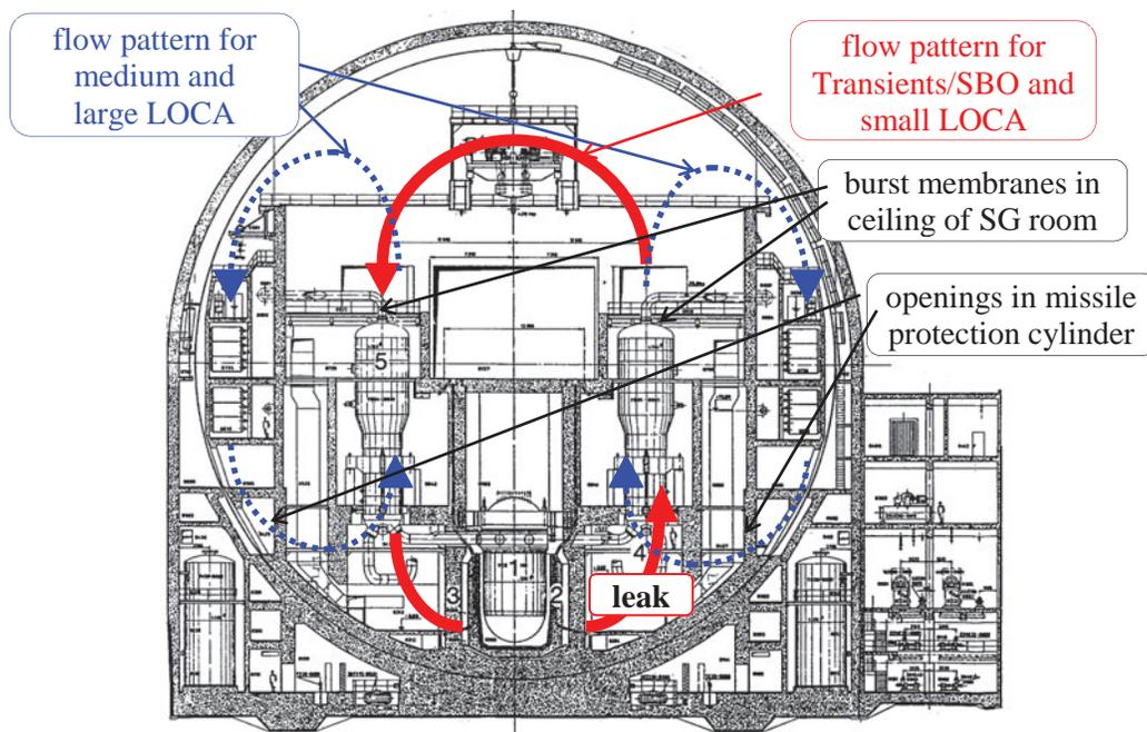
**Figure 1. Main convection flow pattern in German PWR containments.**
