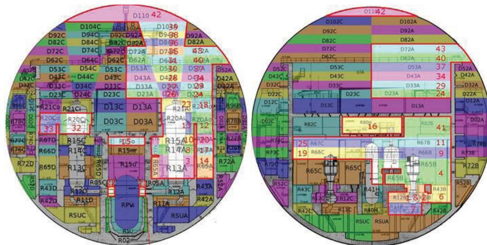
Figure 11. Flame propagation (red numbers from 1-50) through containment (front view and 90° view) with combustion initiated in the cavity, “worst-case” scenario, LB LOCA [10].
