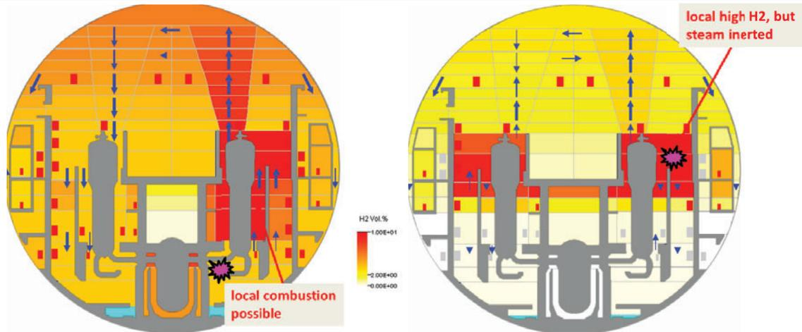
~100 min: LB LOCA; strong short H<sub>2</sub> & steam release due to core relocation into lower plenum; all PARs in operation (red box), combustion -> see chapter 5.3
