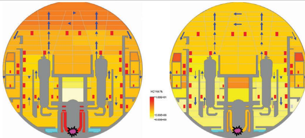
~110 min: LB LOCA; RPV failure, MCCI -> H<sub>2</sub>/CO release, all PARs in operation, slight stratification
