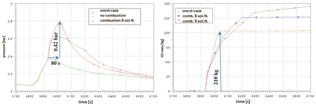
Figure 10. Containment pressure (left) and H<sub>2</sub> mass burned (right) in case of local H<sub>2</sub> combustion initiated at different conditions, LB LOCA [10].
