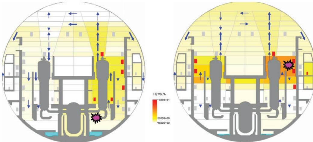
~30 min: LB LOCA; no steam inertisation, start of H<sub>2</sub>-release and PAR operation (red box)
