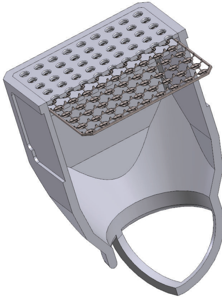
Figure 1 Isometric cut drawing of the lower tie plate including the reverse flow preventer structure
