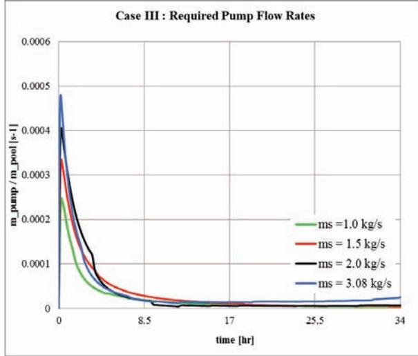
**Figure 11: Series III - GOTHIC Required Pump Flow Rate / Pool Liquid Mass [s<sup>-1</sup>] Predictions**
