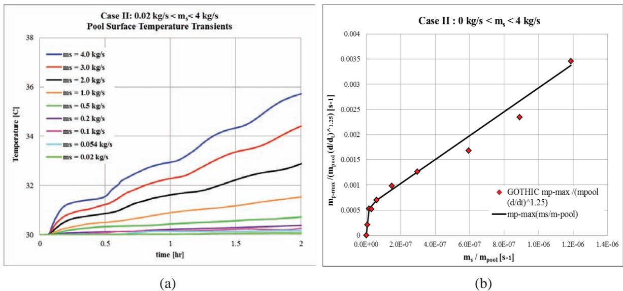
Figure 9: Series II - Surface Temperature Predictions (a) & Maximum Required Mixing Rate (b)
