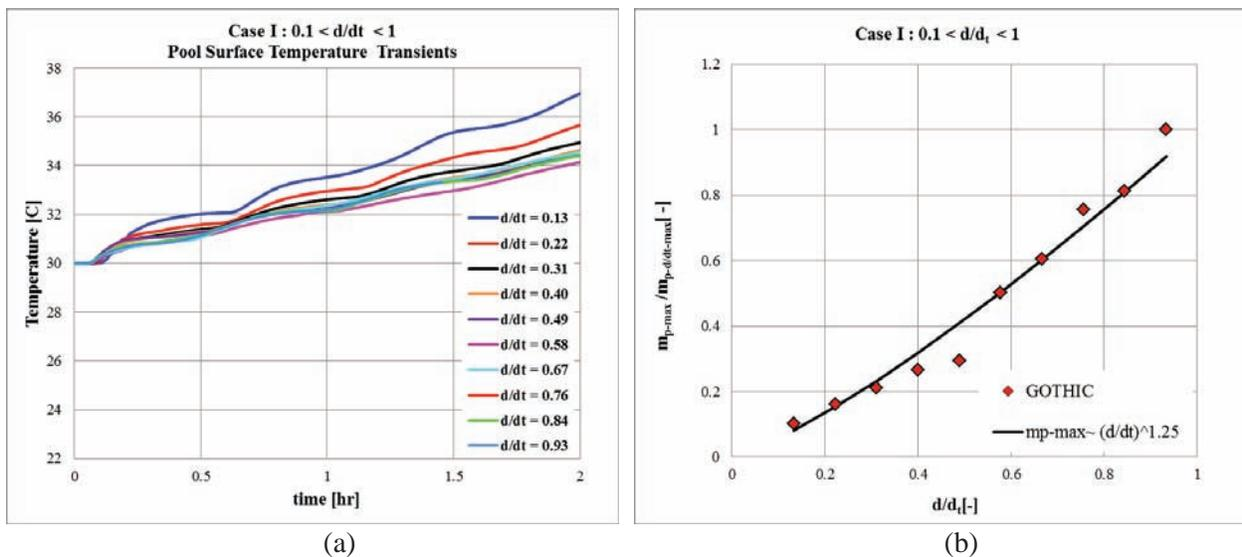
Figure 8: Series I - Surface Temperature Predictions (a) & Maximum Required Mixing Rate (b)
