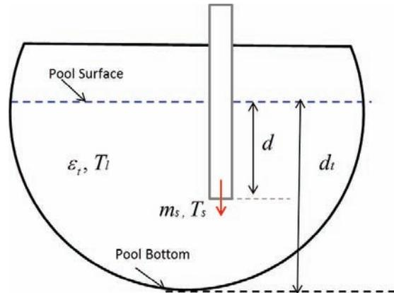
**Figure 7: Suppression Pool Parameters**
