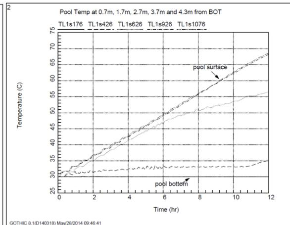
**Figure 3: Suppression Pool Temperature**
