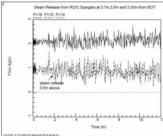
**Figure 4: Steam Release from RCIC Sparger**
