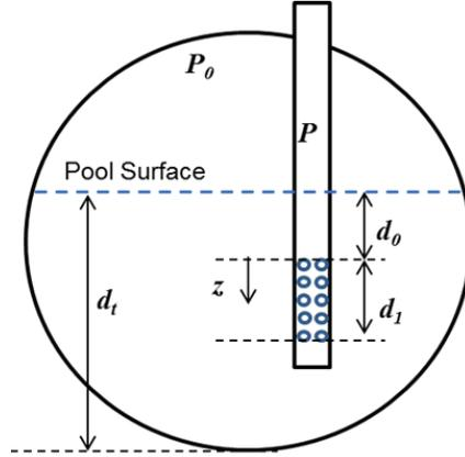
**Figure 10: Suppression Pool Geometric Parameters**
