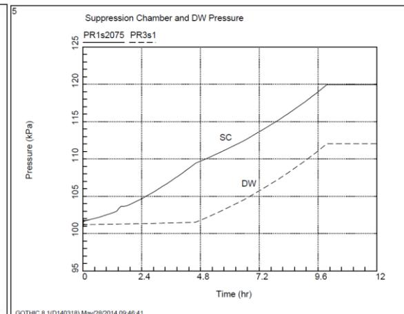
**Figure 5: Torus and Drywell Pressure**
