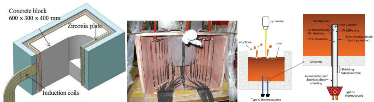
Figure 13. MCCI VULCANO concrete test section
