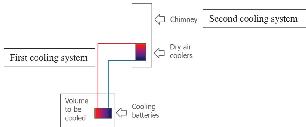
Figure 1. Scheme of the cooling system general structure.
