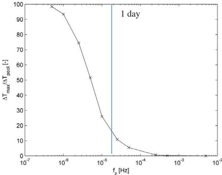
**Figure 3. Passive cooling system frequency response.**
