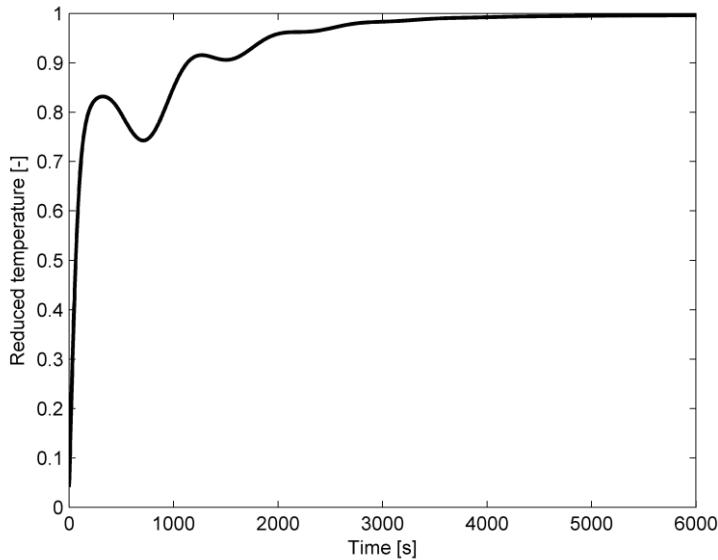
**Figure 5. Hot cell reduced temperature evolution for heat load step.**
