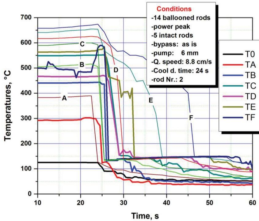
Figure 7. Temperature – time diagram for test CODEX-COOL-24
