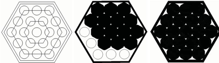
**Figure 1. Cross section of the bundle without sleeves (left) and with 14 (centre) and 19 (right) sleeves in the CODEX-COOL experiments**
