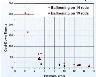
**Figure 2. Cooling-down time dependency in the first 23 CODEX-COOL test**
