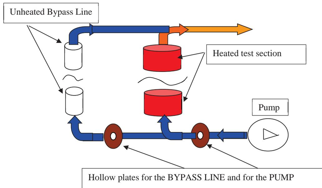
**Figure 4. Understanding the connection of the bypass line**
