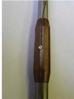
Figure 5. Ballooning simulator (sleeve) on the rod
