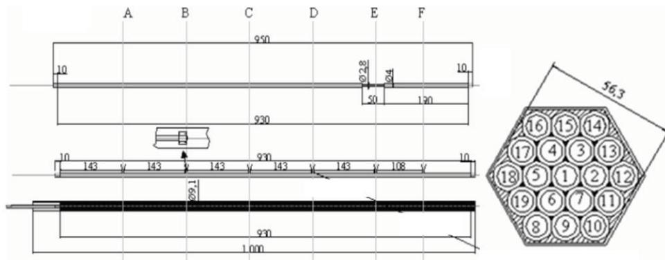
Figure 6. Marked elevations of the thermocouples along the bundle and numbering of the rod simulators
