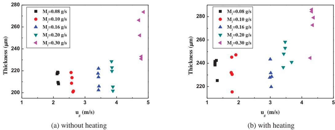
Figure 5. Critical film thickness under different flow conditions
