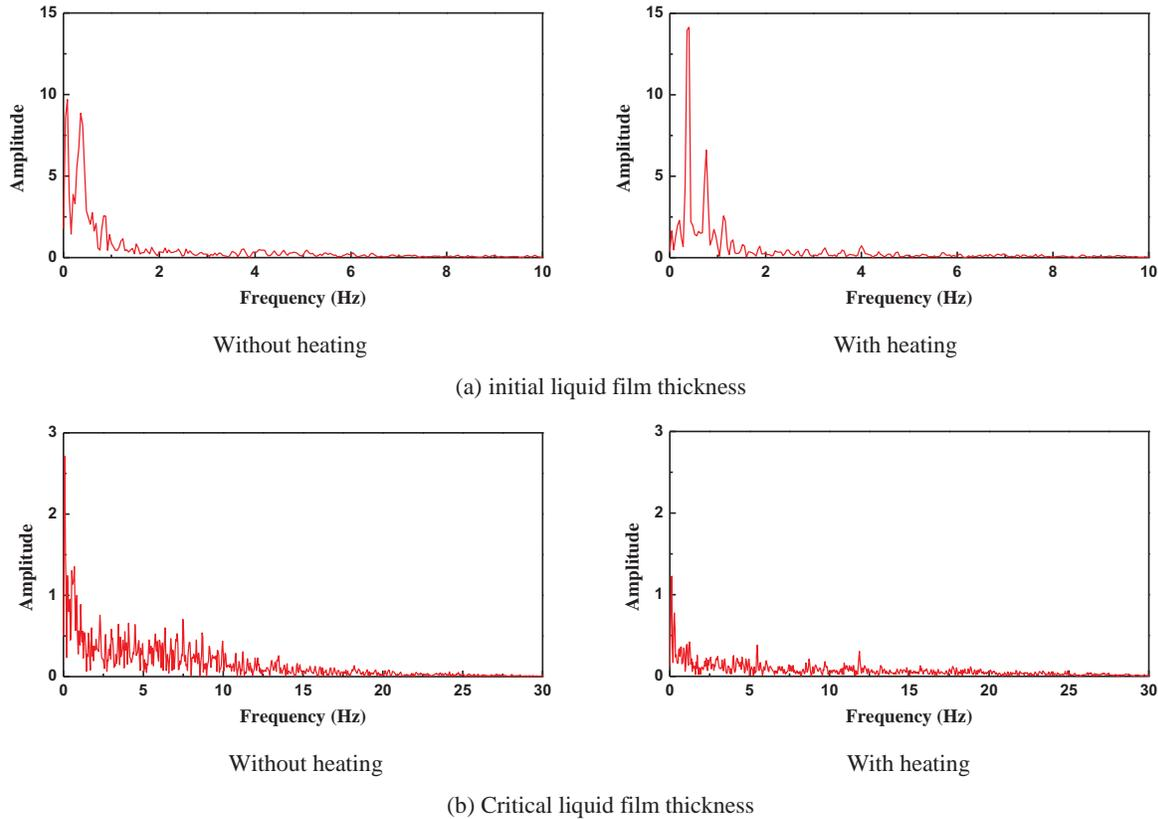
**Figure 9. The effect of heat flux on spectrum of film thickness.**
