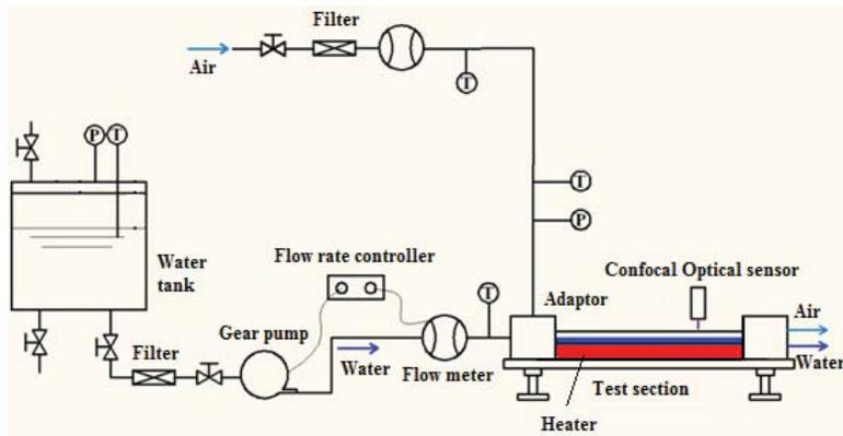
Figure 1. Schematic of test facility.
