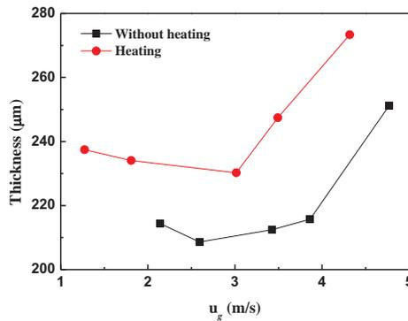
Figure 6. Averaged critical film thickness
