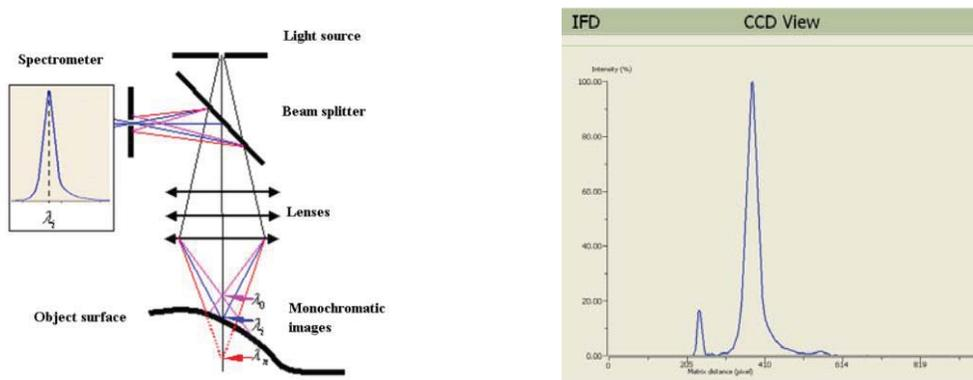
(a) Principle of confocal optical sensor.
