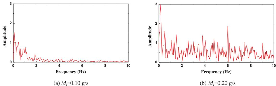
**Figure 8. Spectrum of liquid film thickness under different liquid mass flow rate ( $u_g=2.20$  m/s).**
