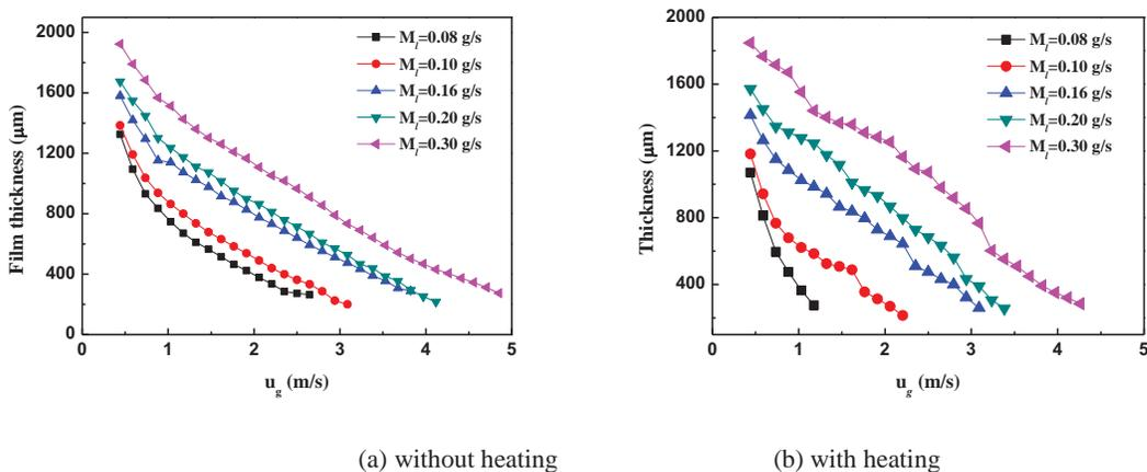
Figure 3. Variation of the liquid film thickness under different flow condition.
