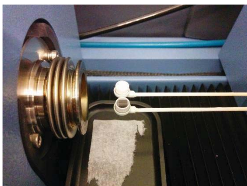
Figure 2 Loaded balance arms in the TGA Apparatus
