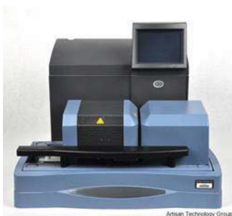
Figure 1 Texas Instruments TGA Apparatus
