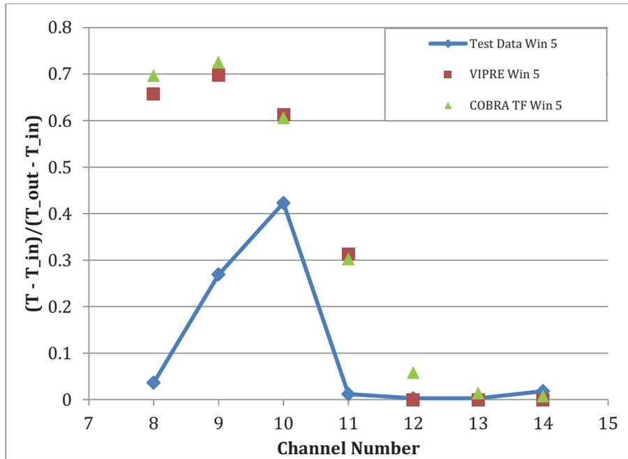
Figure 4. PNNL 2x6: Comparison of Temperature at Window 5 Elevation
