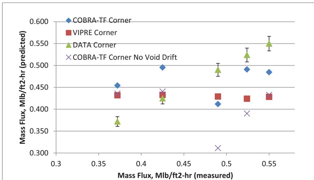
Figure 7. GE 3x3: Comparison of VIPRE and CTF results for GE 3x3 test (corner)
