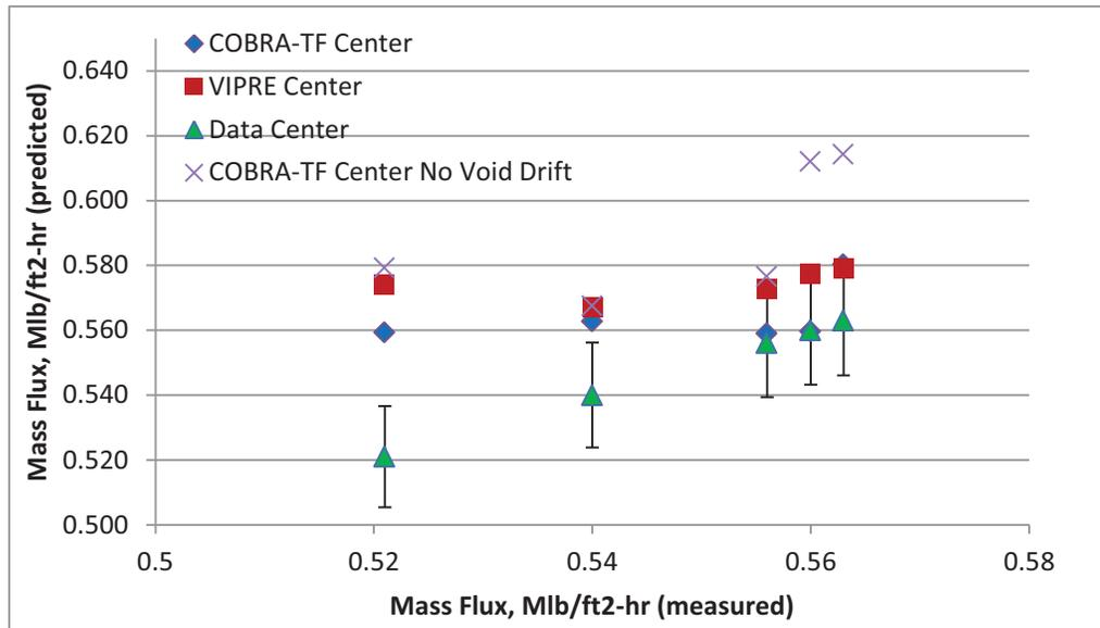
**Figure 8. GE 3x3: Comparison of VIPRE and CTF results for GE 3x3 test (center)**
