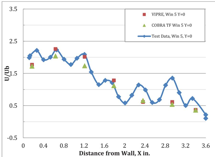
**Figure 3. PNNL 2x6: Comparison of Velocities at Window 5 Elevation**
