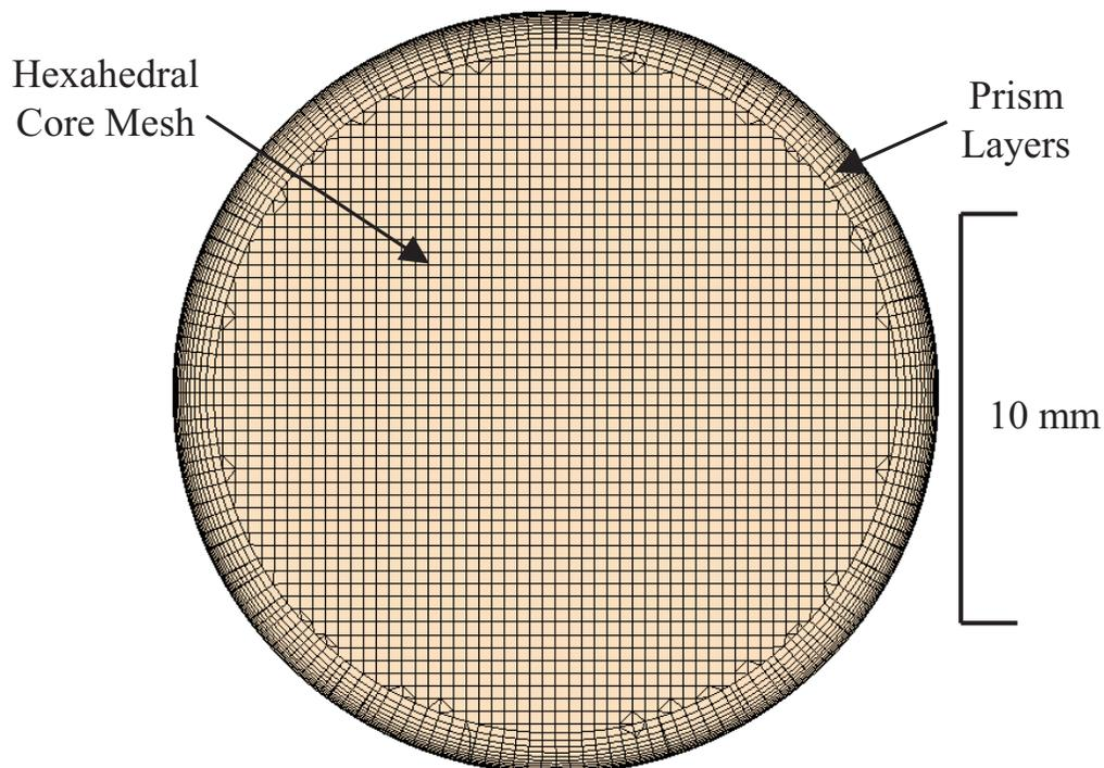
**Figure 4. Cross Sectional Views of the Numerical Meshing Grid used in the CFD Analyses of the Test Section in Fig. 3.**
