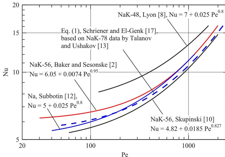
**Figure 1. Thermally Fully-Developed Nu Correlations for Alkali Liquid Metals flow in Uniformly Heated Tubes.**
