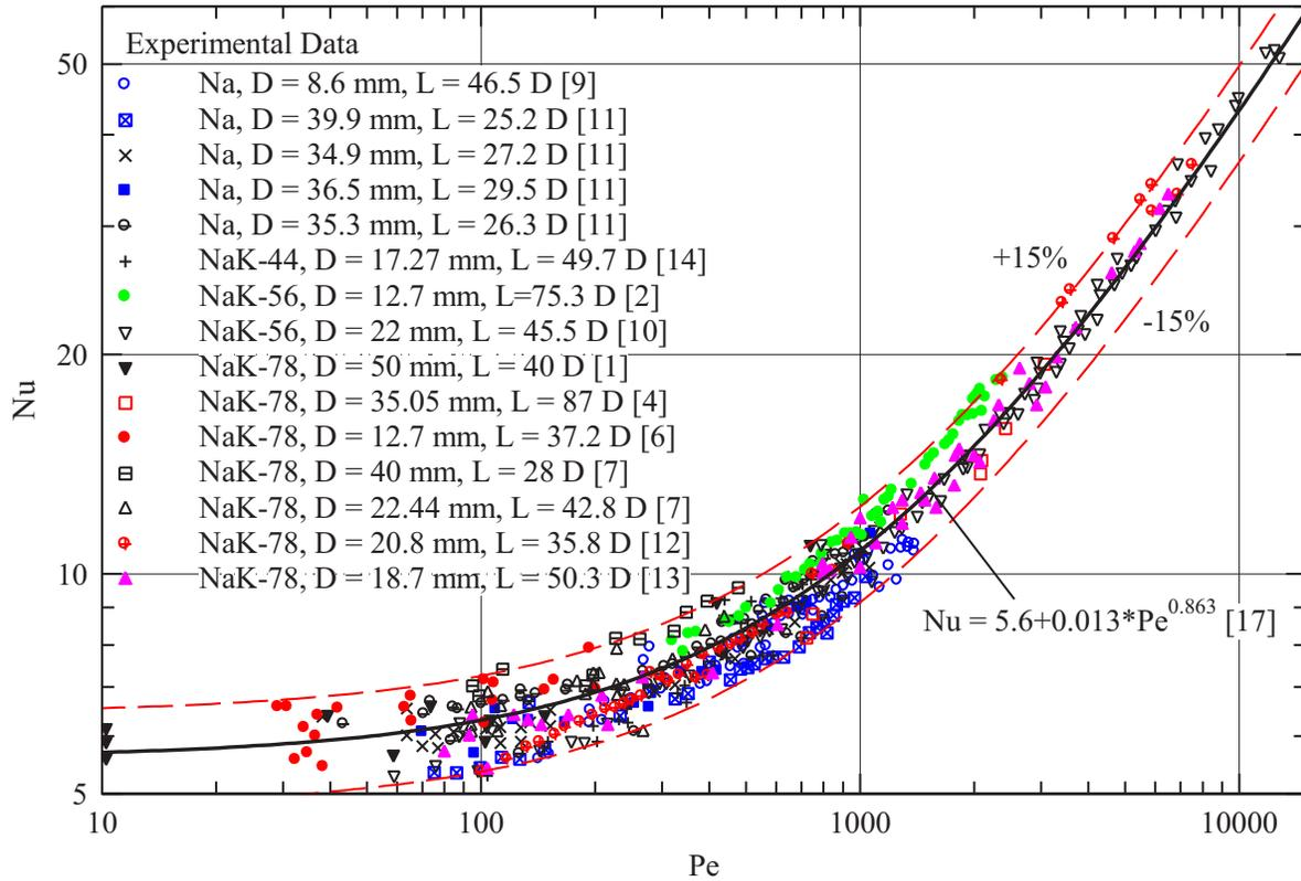
**Figure 2. Comparison of Compiled Data of Thermally Developed Nu for Alkali Liquid Metals Flow in Uniformly Heated Tubes with Correlation [17].**
