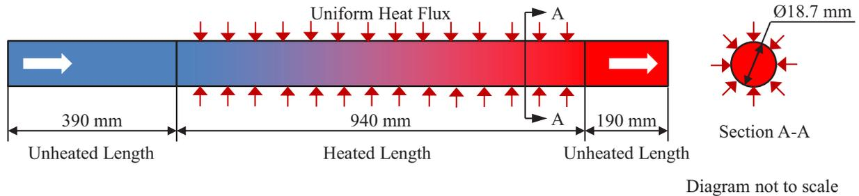
**Figure 3. Test Section in the Experiments of Talanov and Ushakov [13].**
