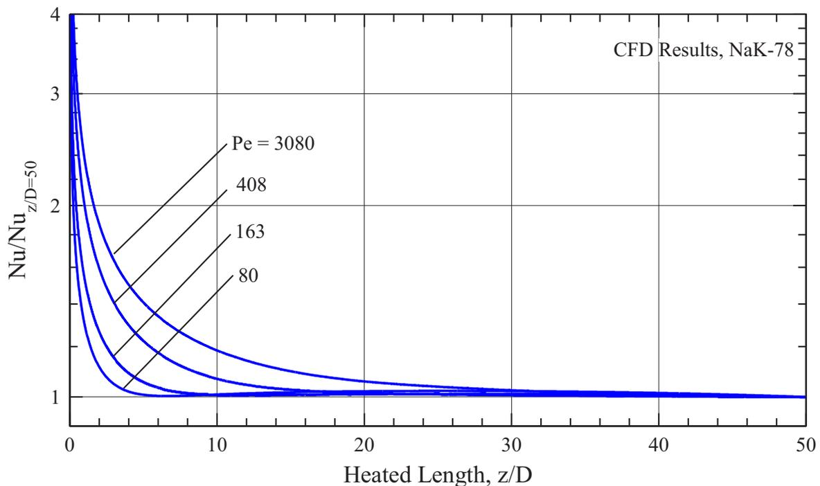
Figure 6. CFD Results of the Local Nu along the Heated Tube Length in the Test Section in Fig. 3, at Different inlet Pe values.
