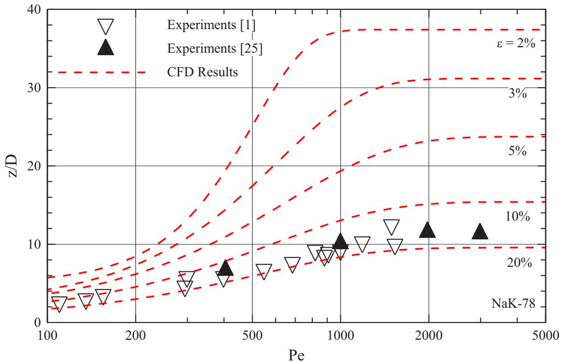
**Figure 7. CFD Results of Convergence of Nu Values to that at the End of the Heated Tube Length in the Test Section in Fig. 3.**
