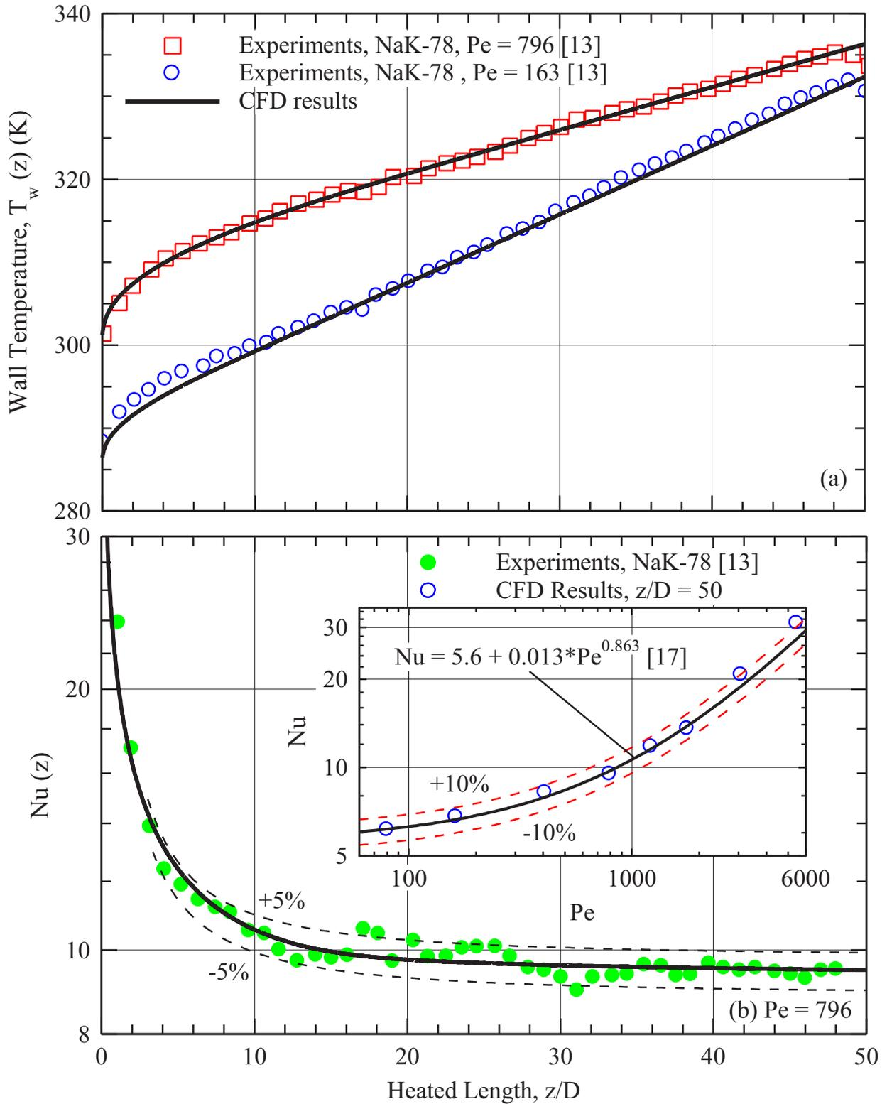
Figure 5. Comparison of Calculated and Experimental Results for NaK-78 Flow in the Heated Tube Length of Test Section in Fig. 3: (a) Axial Wall Temperatures (a), and (b) Local Nu
