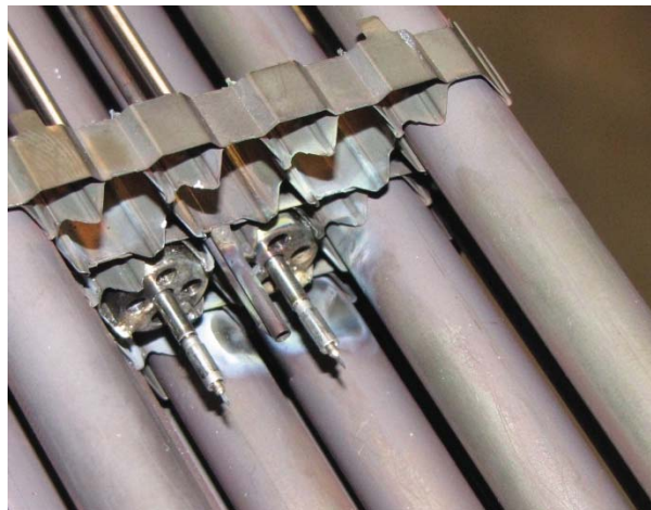
Figure 3. Pitot tube and optical probes installation inside the test bundle (at EOHL)
