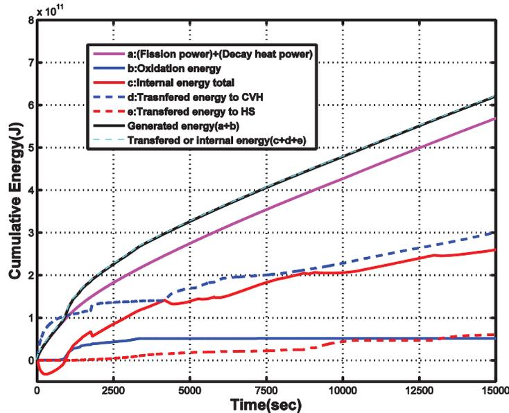
Figure 9. Cumulative energy (generated, internal and transferred energy in the reactor core)
