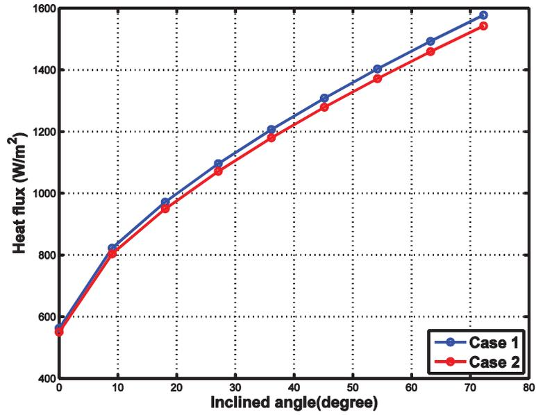
Figure 13. Critical heat flux on the external vessel wall
