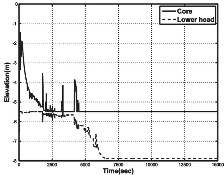
Figure 5. Coolant elevation in the reactor core
