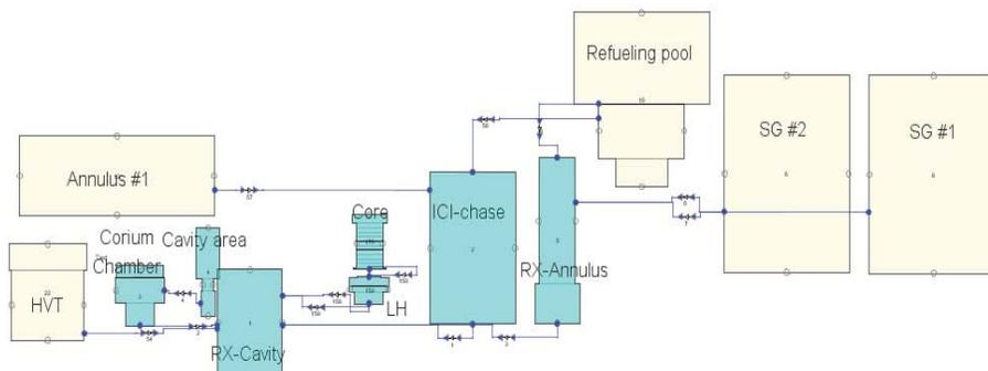
**Figure 3. Flow path between reactor, reactor cavities and other control volumes**
