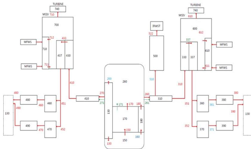
**Figure 1. Schematic of APR1400 RCS MELCOR nodalization**
