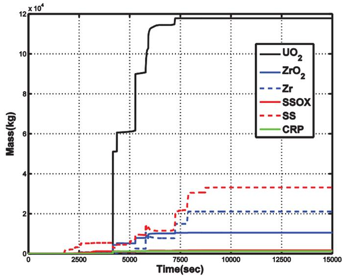
Figure 10. Mass of relocated core materials in the lower plenum
