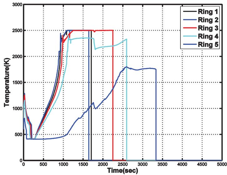
Figure 8. Temperature of fuel cladding (at axial level 13)
