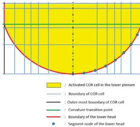
**Figure 2. Core cell and lower head nodalization in the lower plenum**
