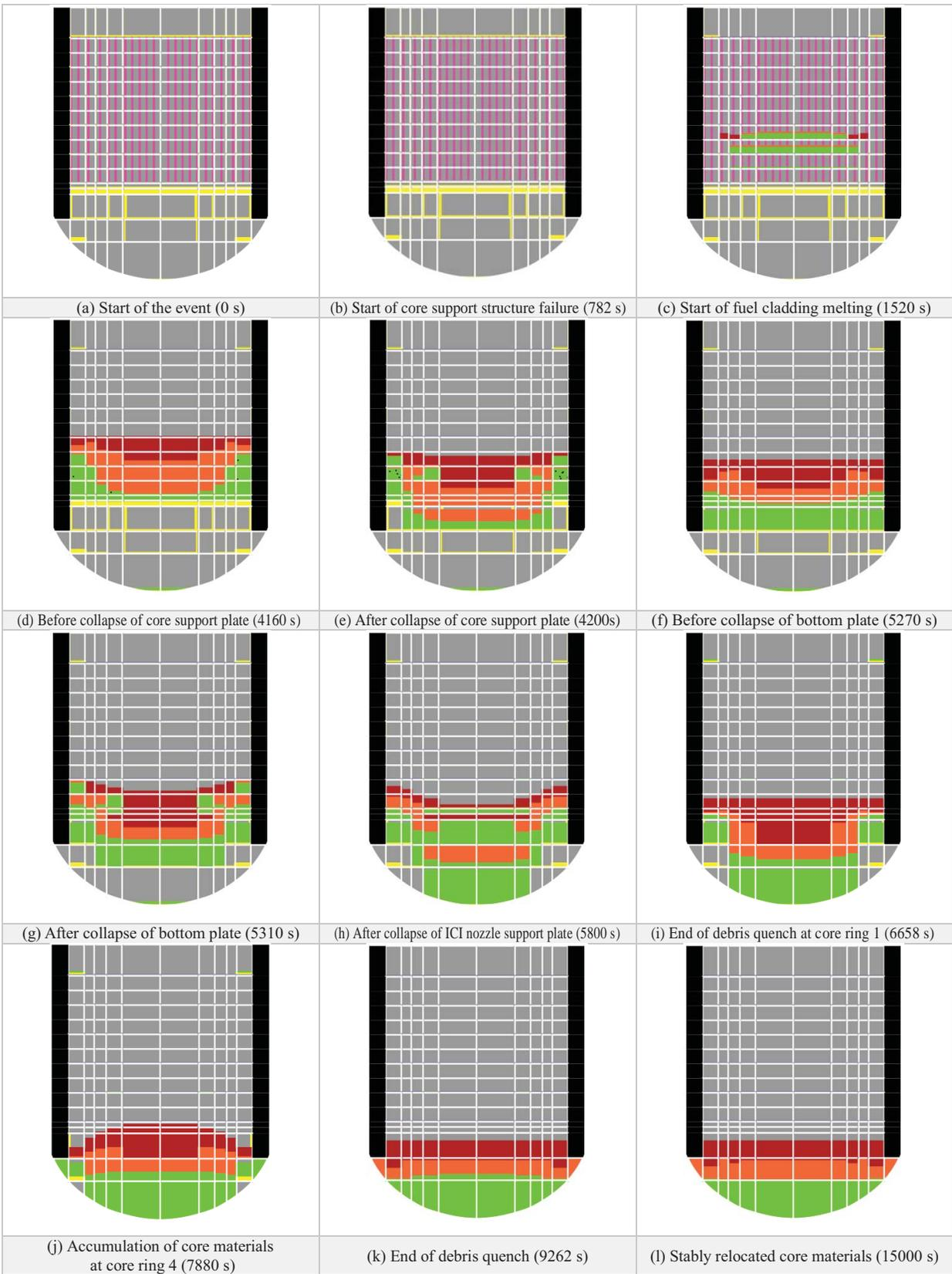
**Figure 4. Core degradation behavior**
