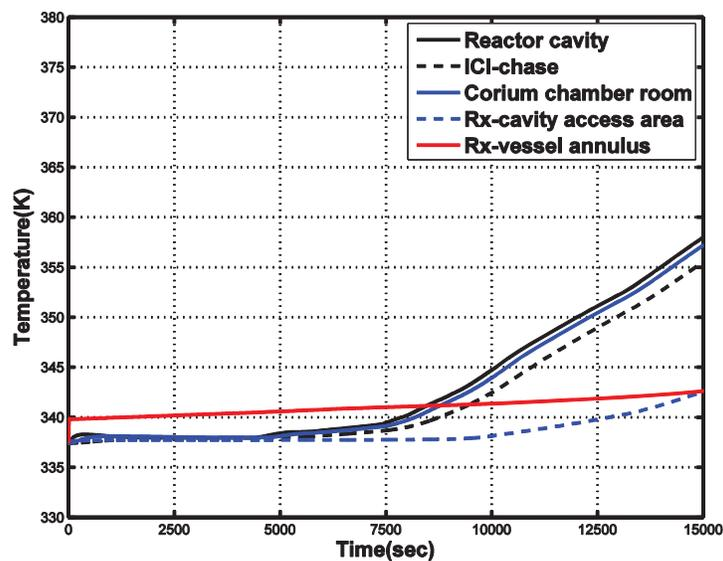
Figure 6. Temperature of the reactor cavity
