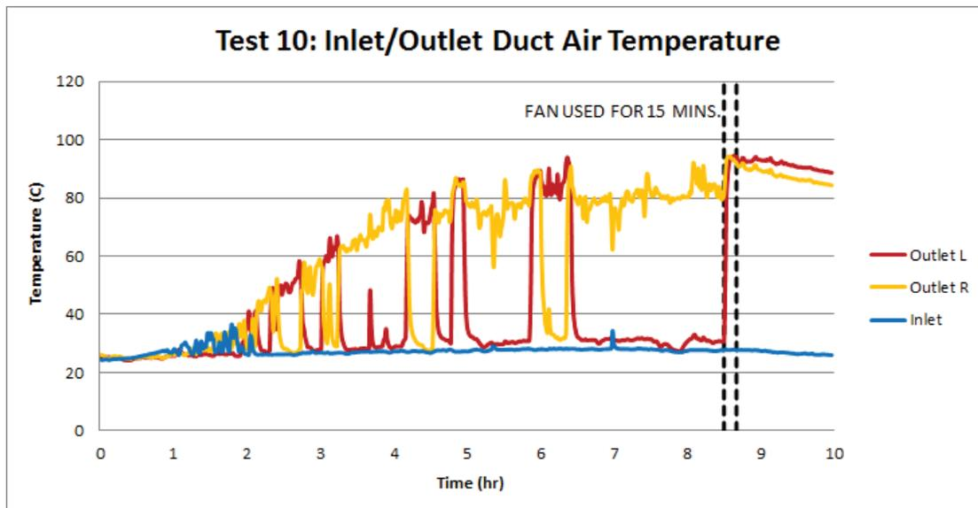
Figure 14 – Inlet and exhaust duct air temperature for Test 10 (Uncertainty:  $\pm 0.7^{\circ}\text{C}$ ).
