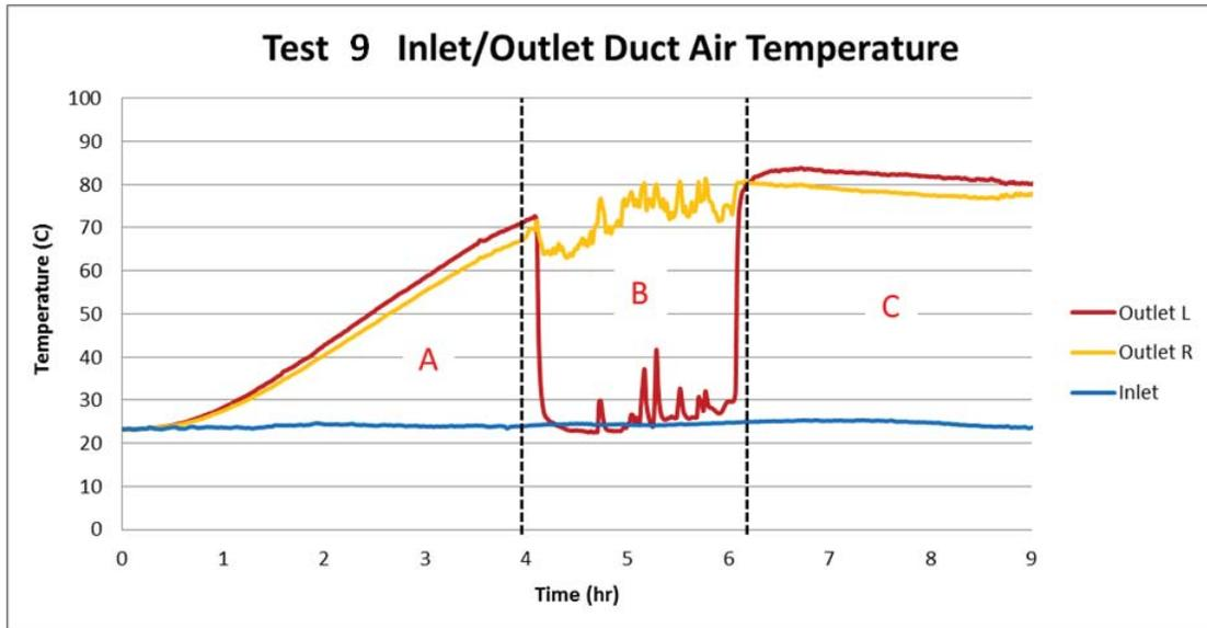
Figure 12 – Inlet and exhaust duct air temperature for Test 9 (Uncertainty:  $\pm 0.7^{\circ}\text{C}$ ).
