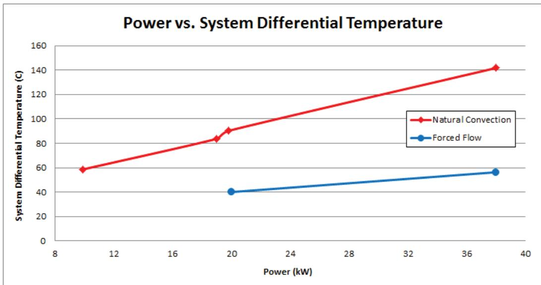
Figure 18 – System differential temperatures for all test conditions.
