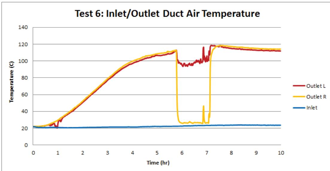
Figure 8 – Inlet and exhaust duct air temperature for Test 6 (Uncertainty:  $\pm 0.7^{\circ}\text{C}$ ).
