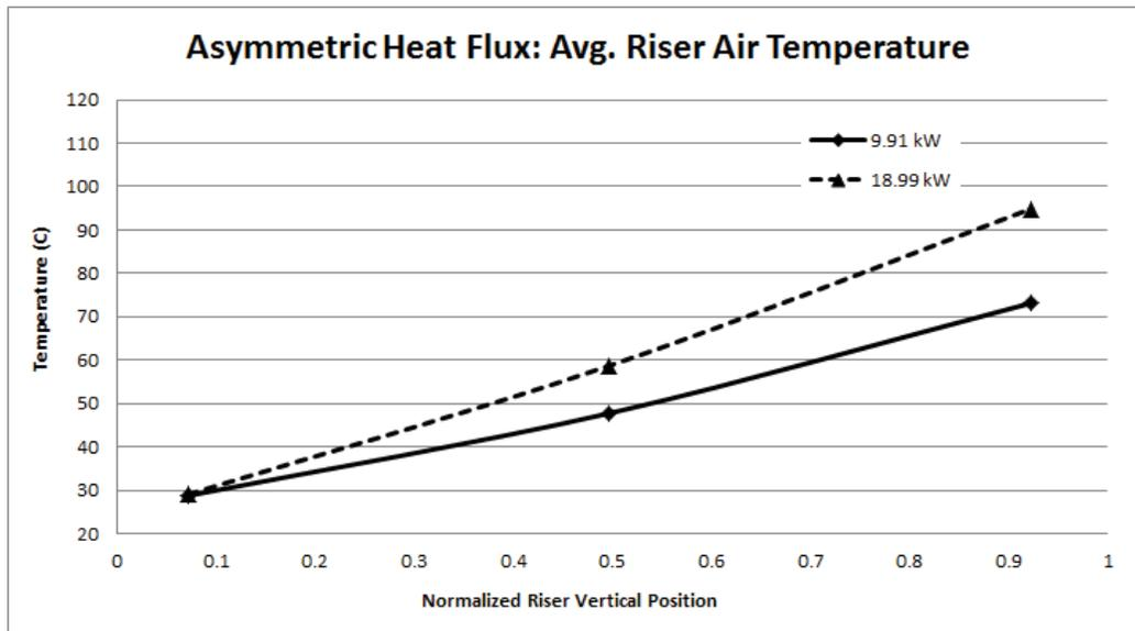
Figure 11 - Riser air temperatures for forced flow (Uncertainty:  $\pm 0.7^\circ\text{C}$ ).
