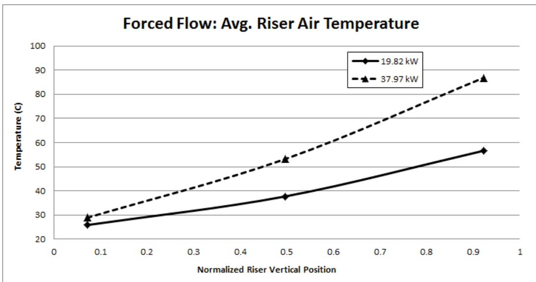
Figure 5 - Riser air temperatures for forced flow (Uncertainty:  $\pm 0.7^{\circ}\text{C}$ ).
