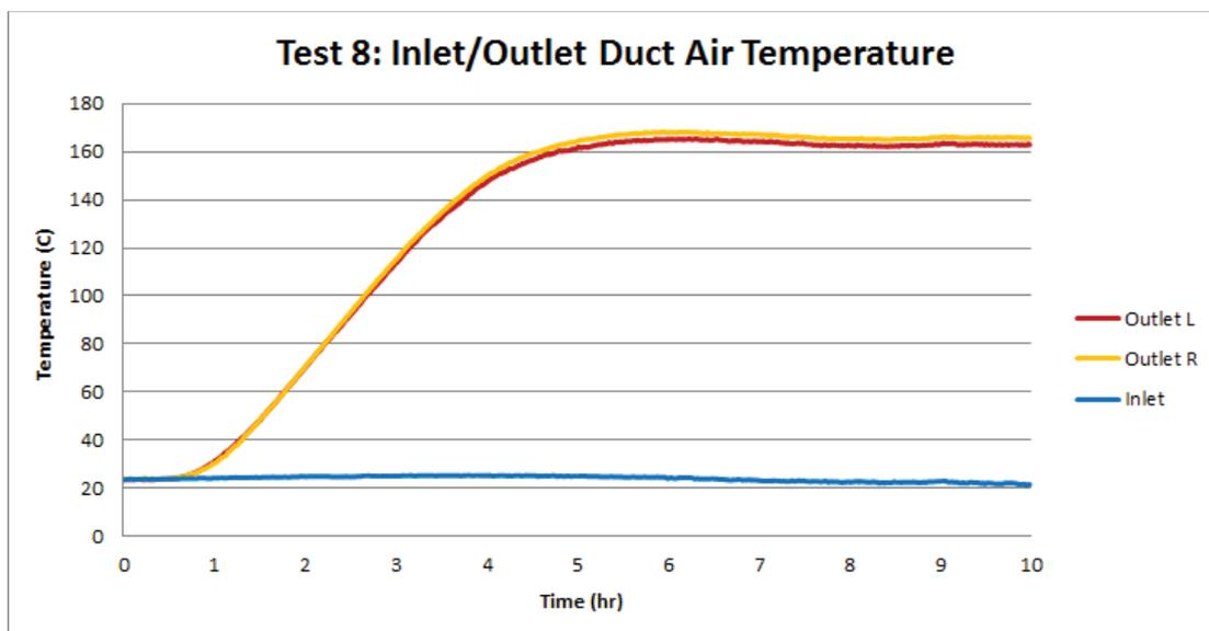
Figure 10 – Inlet and exhaust duct air temperature for Test 8 (Uncertainty:  $\pm 0.7^{\circ}\text{C}$ ).
