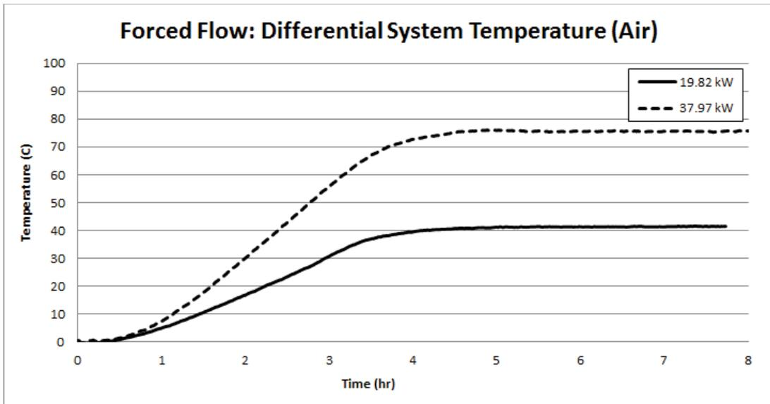
Figure 4 – Differential system temperature (air) for forced flow (Uncertainty:  $\pm 0.7^{\circ}\text{C}$ ).
