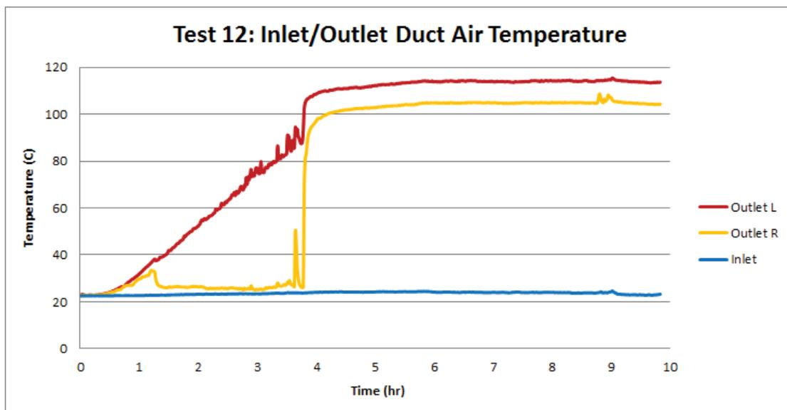
Figure 17 – Inlet and exhaust duct air temperature for Test 12 (Uncertainty:  $\pm 0.7^{\circ}\text{C}$ ).
