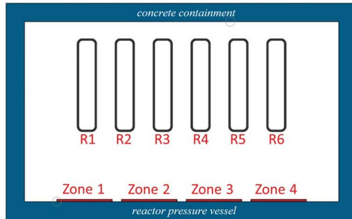
Figure 3 – Heated cavity section view.
