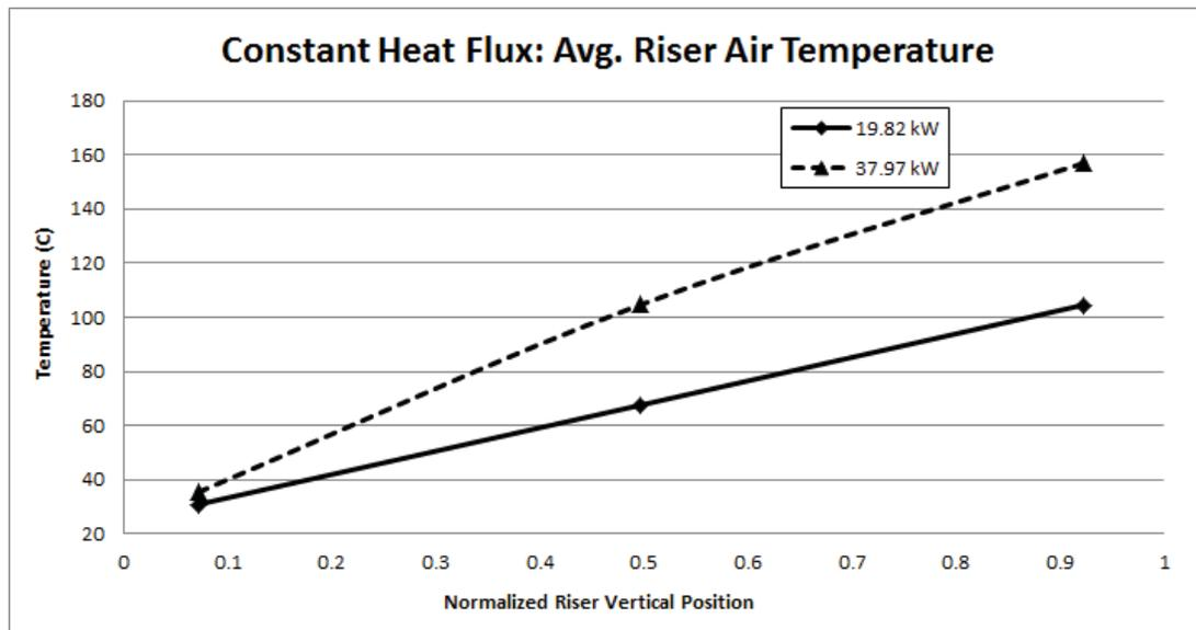
Figure 6 - Riser air temperatures for forced flow (Uncertainty:  $\pm 0.7^\circ\text{C}$ ).
