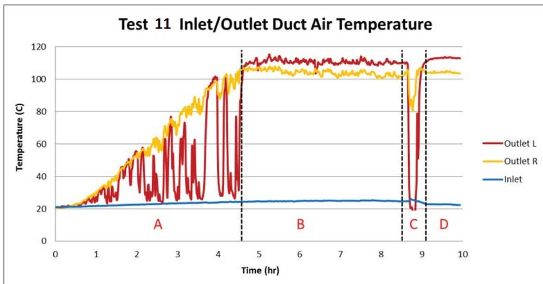
Figure 15 – Inlet and exhaust duct air temperature for Test 11 (Uncertainty:  $\pm 0.7^{\circ}\text{C}$ ).
