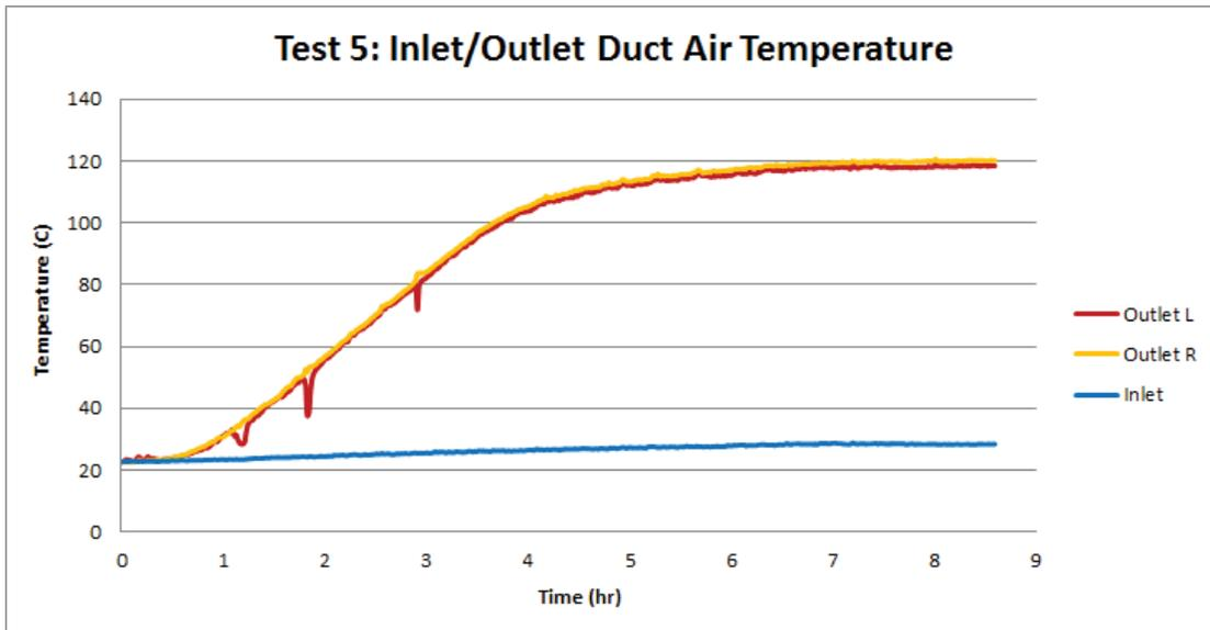
Figure 7 – Inlet and exhaust duct air temperature for Test 5 (Uncertainty:  $\pm 0.7^{\circ}\text{C}$ ).
