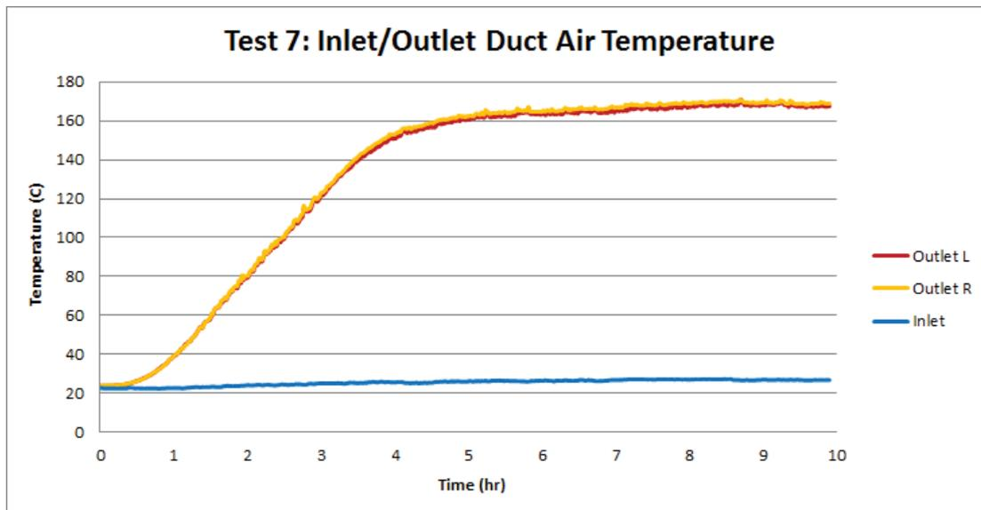
Figure 9 – Inlet and exhaust duct air temperature for Test 7 (Uncertainty:  $\pm 0.7^{\circ}\text{C}$ ).
