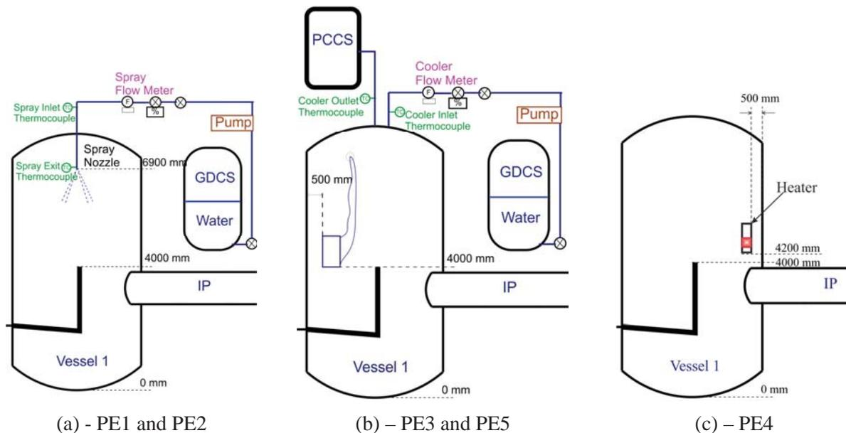
Figure 1. Experimental set-ups for (a)-spray (b)-cooler and (c)-heater device tests.
