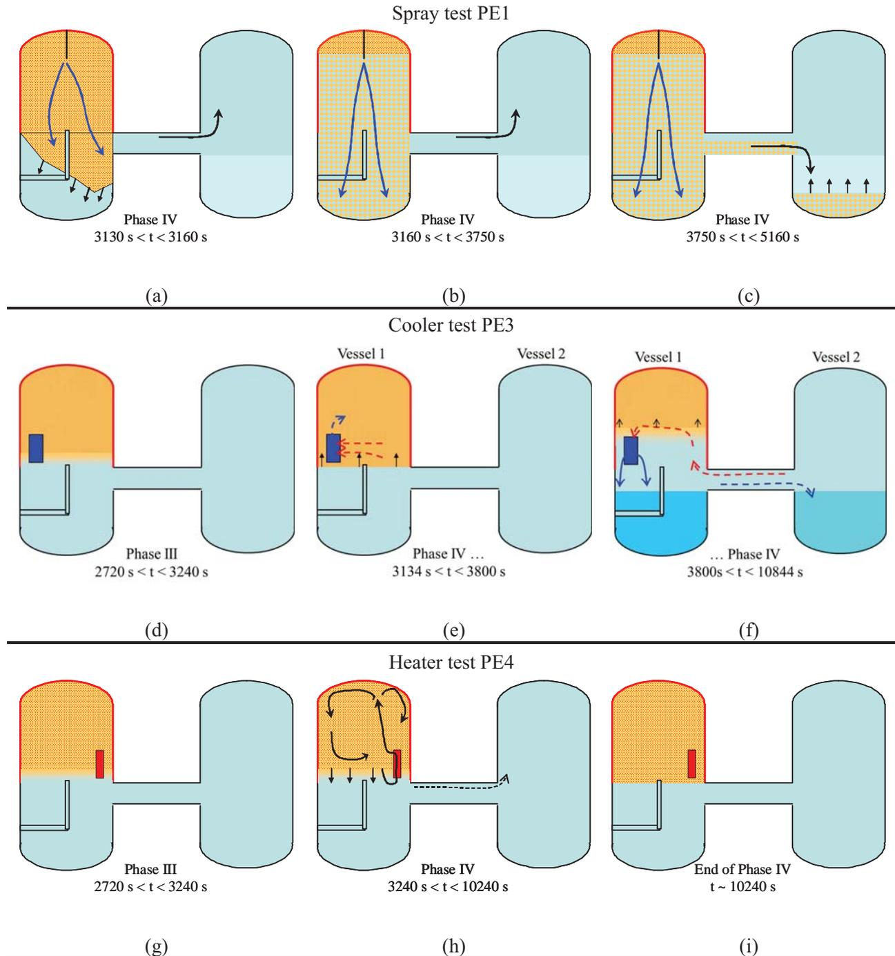
**Figure 12. Flow patterns observed during the activation of the safety system in phase IV for test PE1, PE3 and PE4.**
