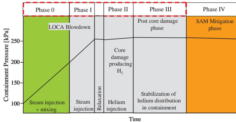
**Figure 2. Schema of representing the test scenario followed during the PANDA experiments**
