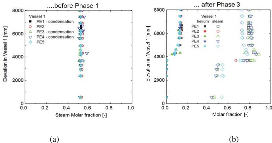
**Figure 3. (a)Initial steam concentration and (b) intermediate steam/helium concentration vertical profile before activation of safety system for all five tests.**
