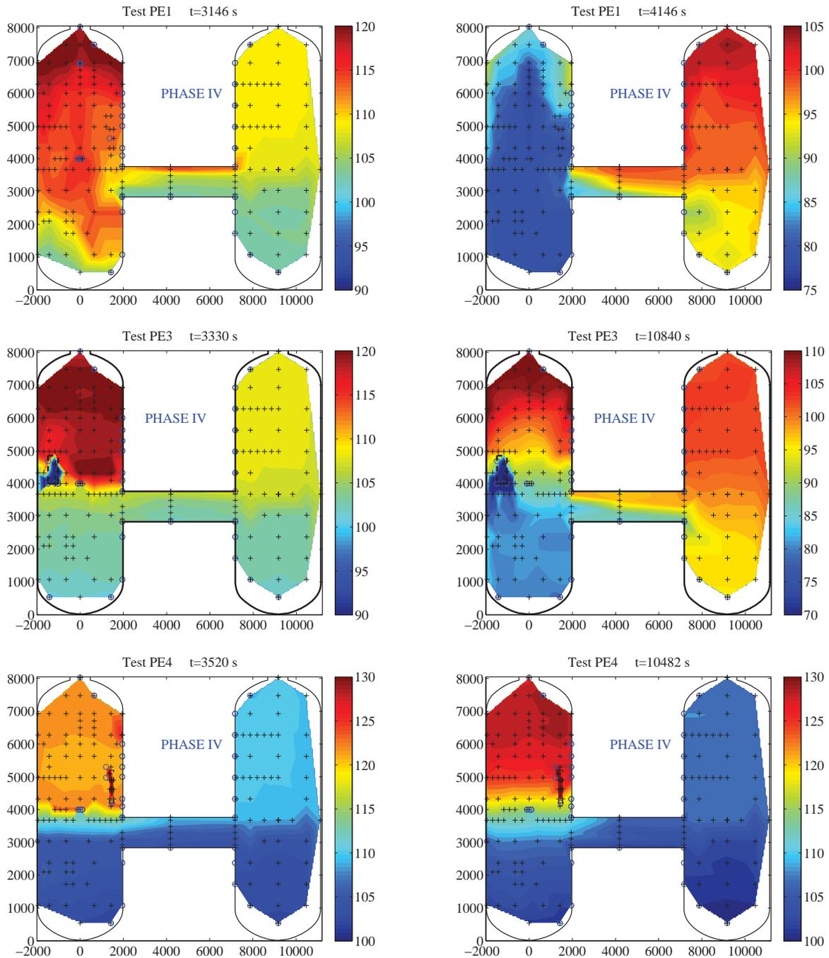
**Figure 9. Selected temperature contour maps representing temperature distribution in vertical plane at the beginning (left side) and at the end (right side) of Phase IV for test PE1, PE3 and PE4.**
