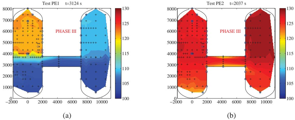
Figure 6. Temperature contour map representing temperature distribution at the end of Phase III for (a) condensing environment PE1 test and (b) non-condensing environment PE2 test.
