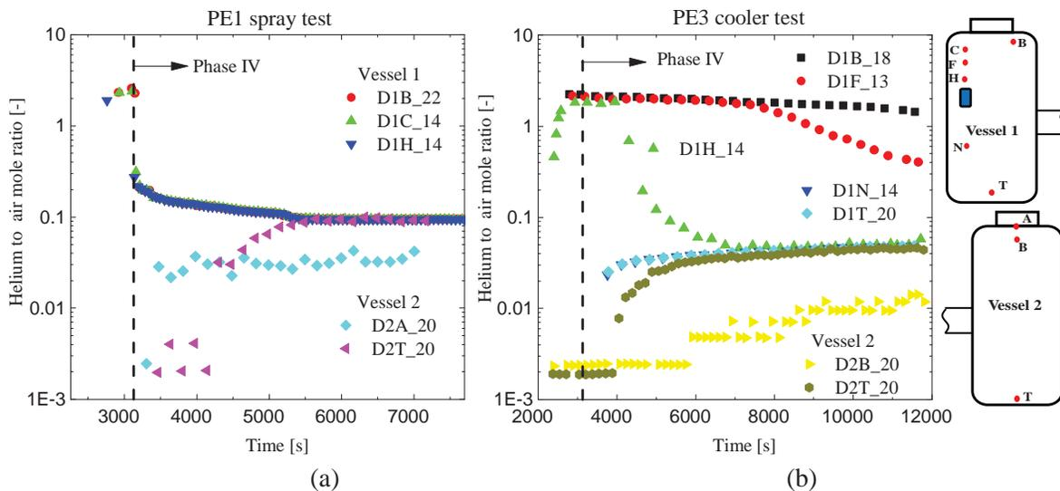
Figure 11. Helium to air mole ratio content at selected position for test -(a) PE1 and -(b) PE3.
