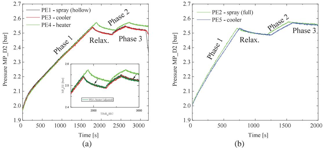
Figure 4. Pressure evolution in Phases I to III for (a) PE1, PE3 and PE4 and (b) PE2 and PE5 tests
