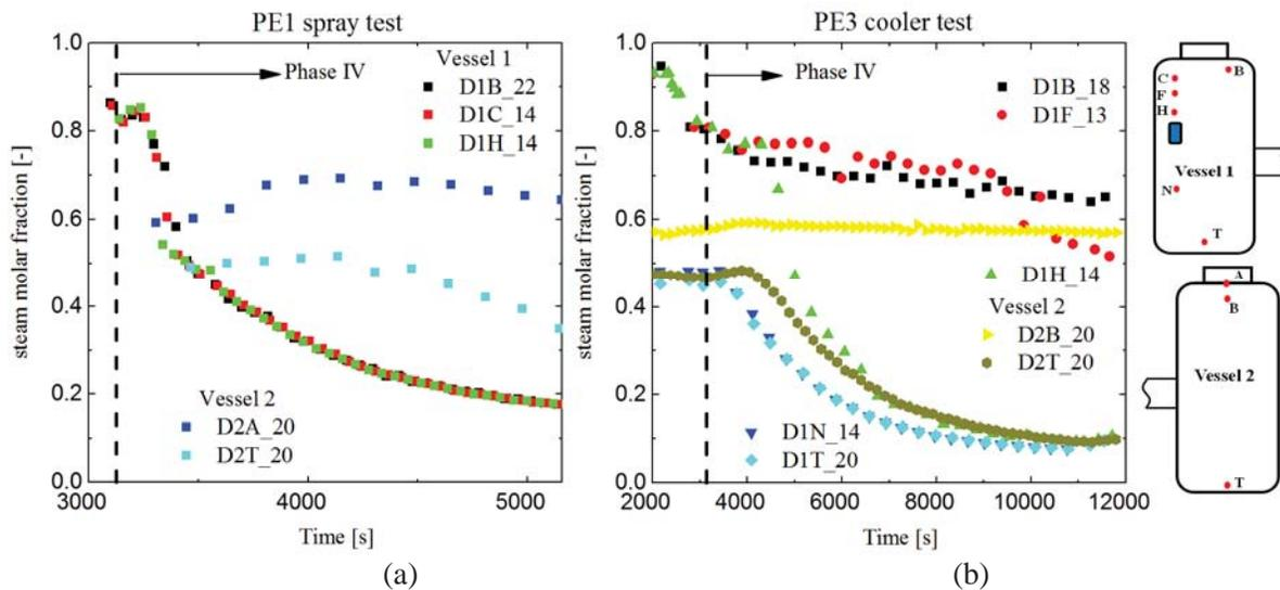
Figure 10. Steam content at selected position for test -(a) PE1 and -(b) PE3.
