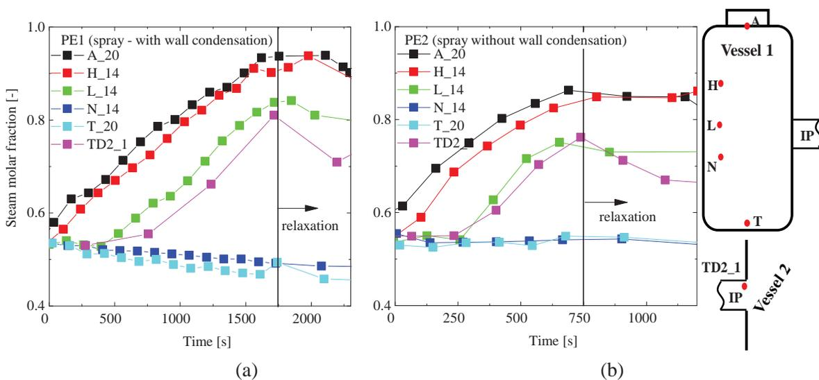
Figure 5. Steam concentration evolution in Phase 1 for test PE1 (left) and PE2 (right).
