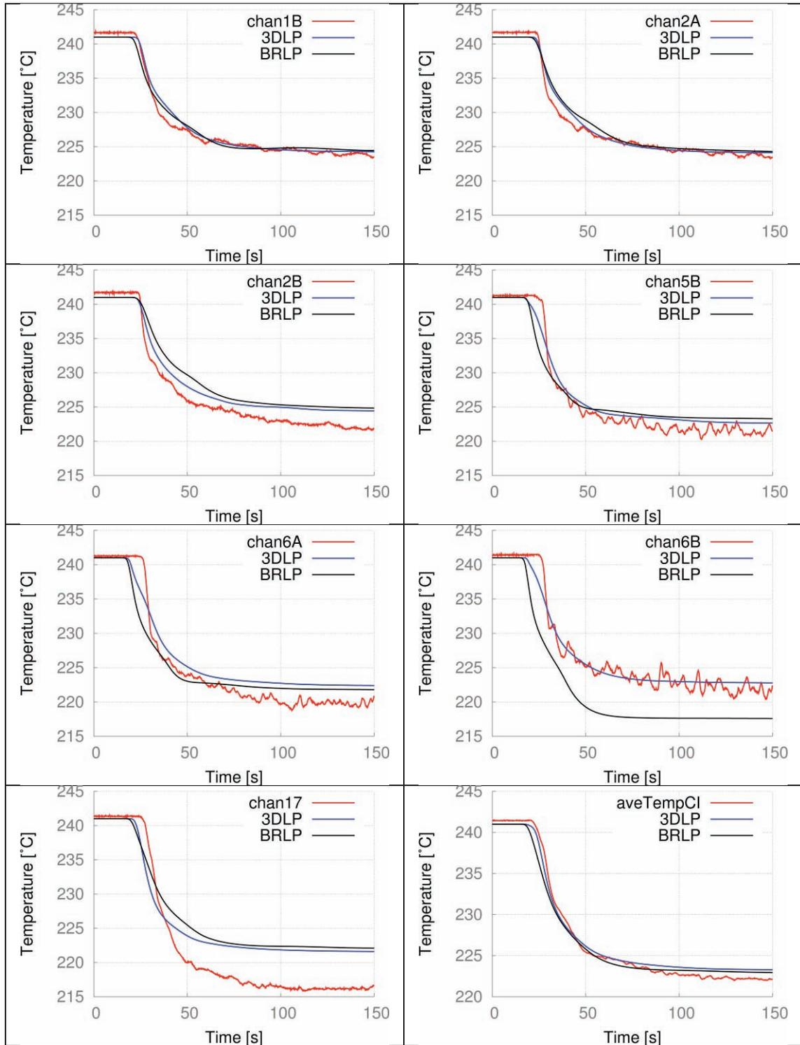
**Figure 6. Temperature trends at the CI for representative core channels and average CI temperature.**
