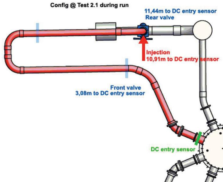
**Figure 2. Configuration of loop 1 (affected loop) during the ROCOM experiment 2.1 [1].**
