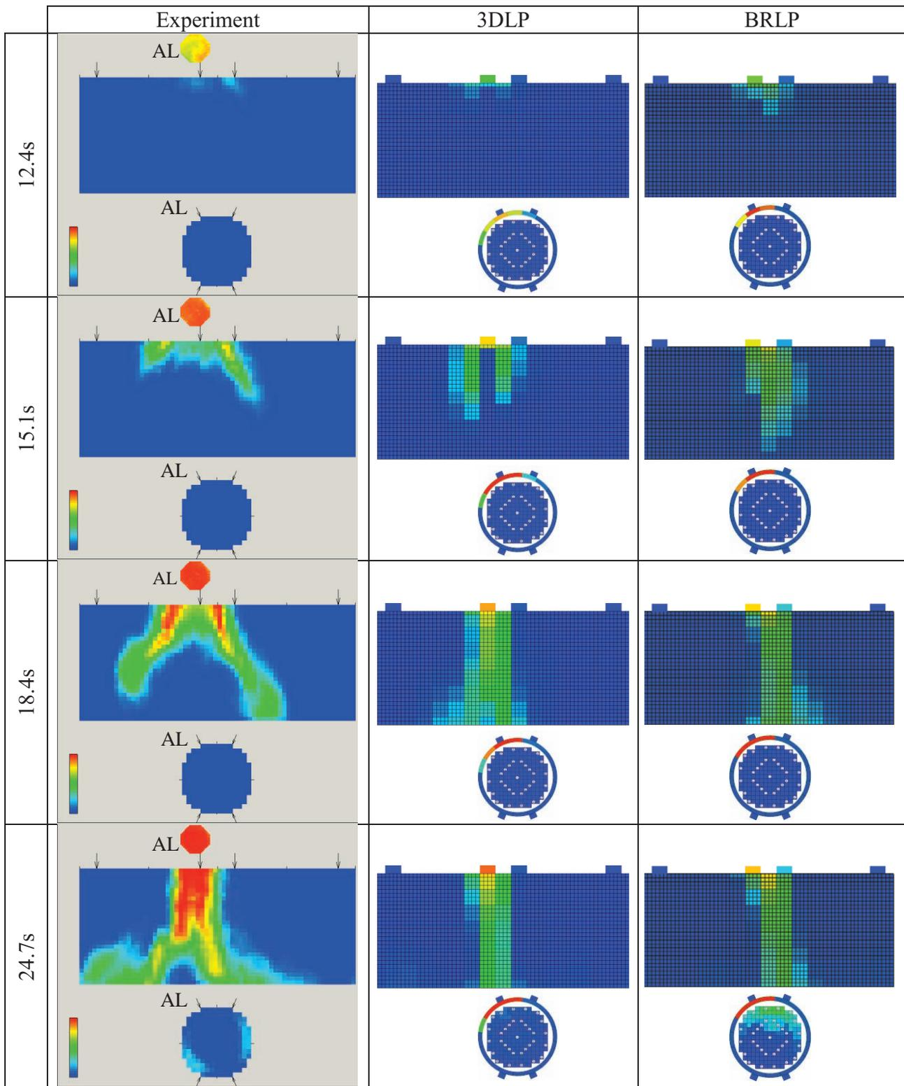
Figure 7. Comparison of the temperature fields derived from measured data and simulated by means of the 3DLP and BRLP models, in the DC and at the CI at temporal key points of the experiment (PT 12.4s to 24.7s).
