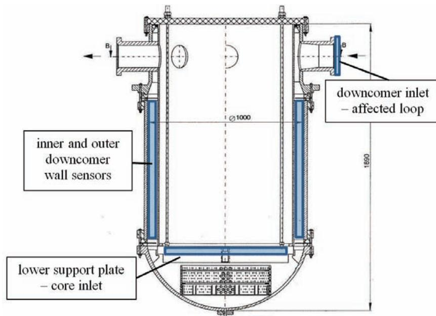
**Figure 1. RPV of the ROCOM facility with the installed WMS [1].**
