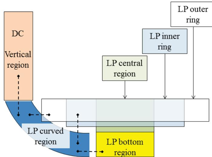
Figure 3. Schematic representation of nodalization employed in the LP
