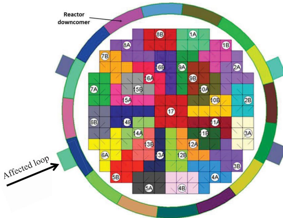
**Figure 4. Schematic drawing of the ATHLET sixteen azimuthal CV representation of the DC and the thirty-three core channels.**
