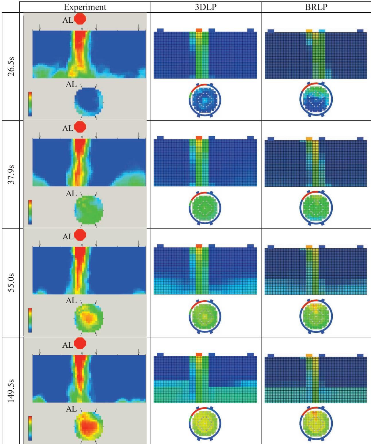
Figure 8. Comparison of the temperature fields derived from measured data and simulated by means of the 3DLP and BRLP models, in the DC and at the CI at temporal key points of the experiment (PT26.5s to 149.5s).
