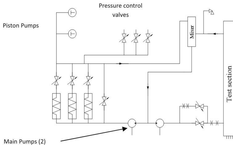
**Figure 1. Schematic of ODEN Loop**
