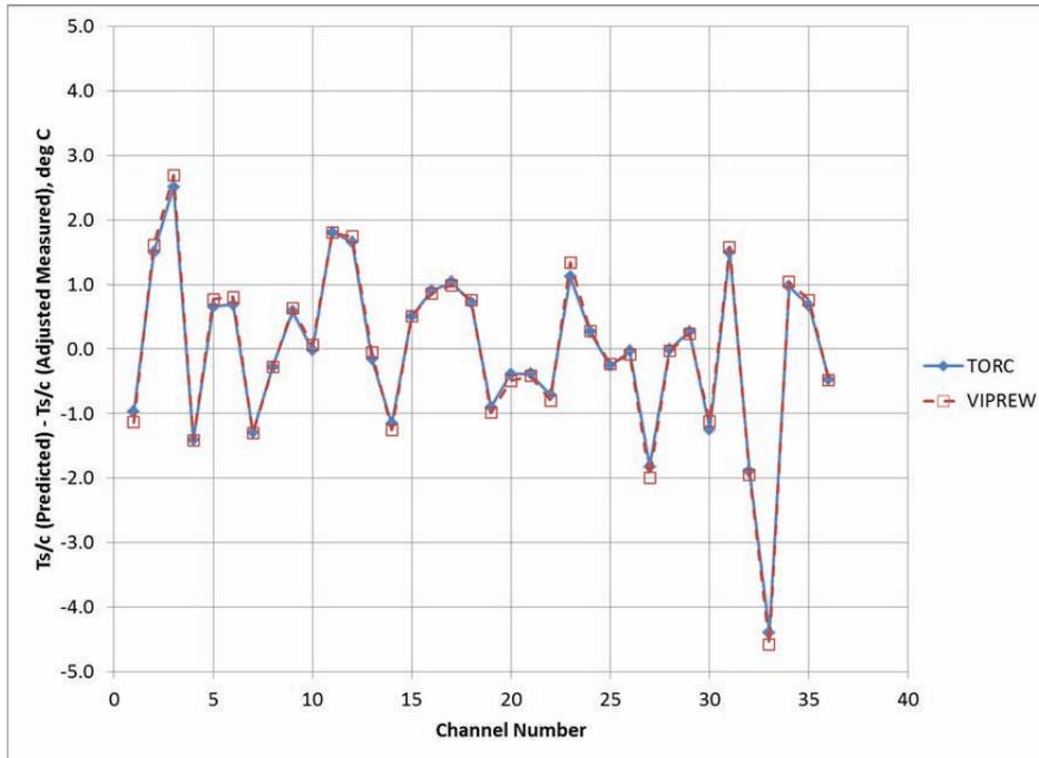
Figure 4. Predicted Minus Measured Subchannel Temperature by Method
