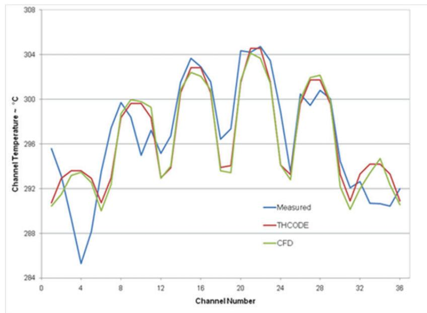
**Figure 3. Example of Sub-Channel Temperatures in a Mixing Test [5]**
