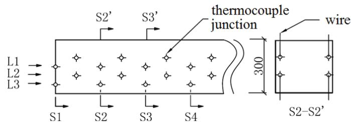
**Figure 10. Thermocouple location and its wire**
