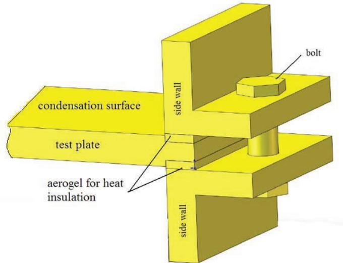
Figure 6. Test plate isothermal method
