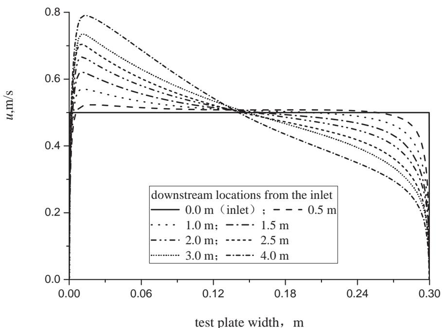
**Figure 4. Velocities of different locations from the test plate entrance**
