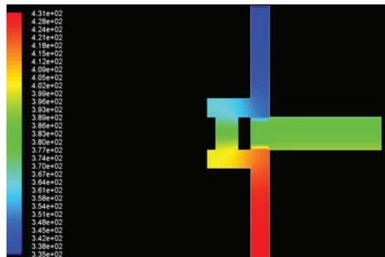
Figure 7. Temperature distributions of the connecting cross-section
