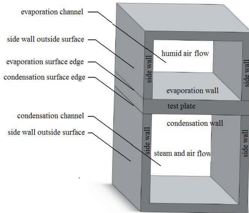
Figure 3. Crossing section of the condensation-evaporation test section
