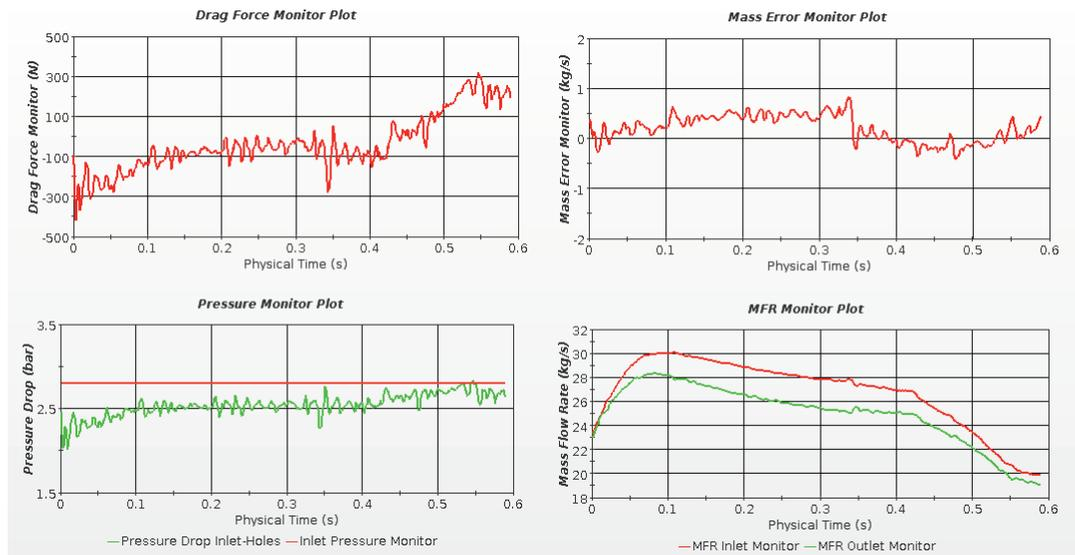
Figure 8: Results of the transient simulation with seal almost conform for 0.6 s of motion
