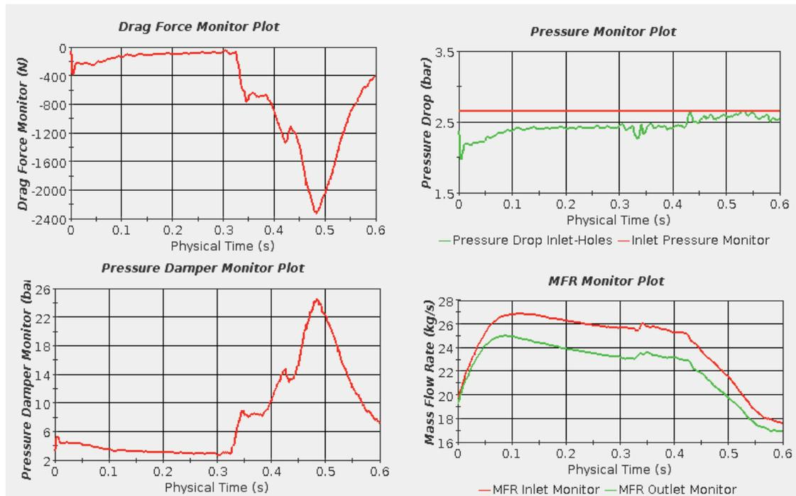
Figure 11: Plots at the end of the insertion in the case with increased viscosity
