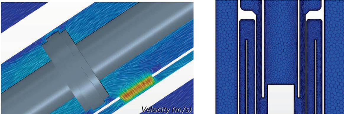
Figure 5: Left, seal almost conform, 2.5 mm of gap to the damper. Right, volume mesh 9 M Cells
