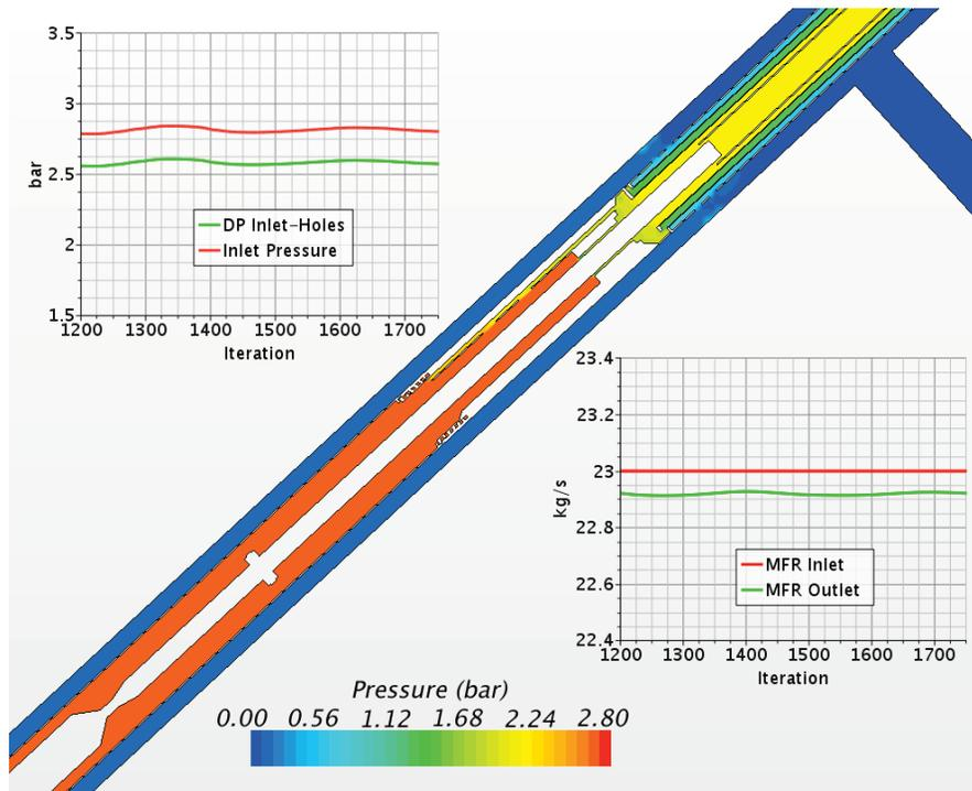
**Figure 6: Steady state results in model with simplified bundle and overlapping grids**
