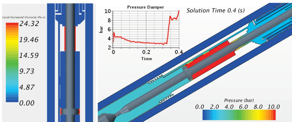
Figure 9: Left, volumes with four orders of magnitude increased viscosity. Right, overpressure due to the seal "sliding" on the damper, compressing the LBE
