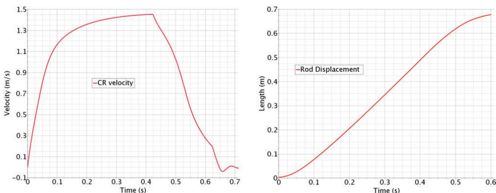
**Figure 7: Imposed displacement, provided by integrated transient accelerations**
