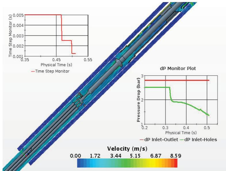
**Figure 4: Motion with almost no influence of the re-meshing on the pressure field**
