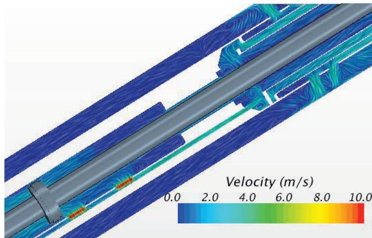
Figure 10: High velocity reached by the LBE flow at the damper slots
