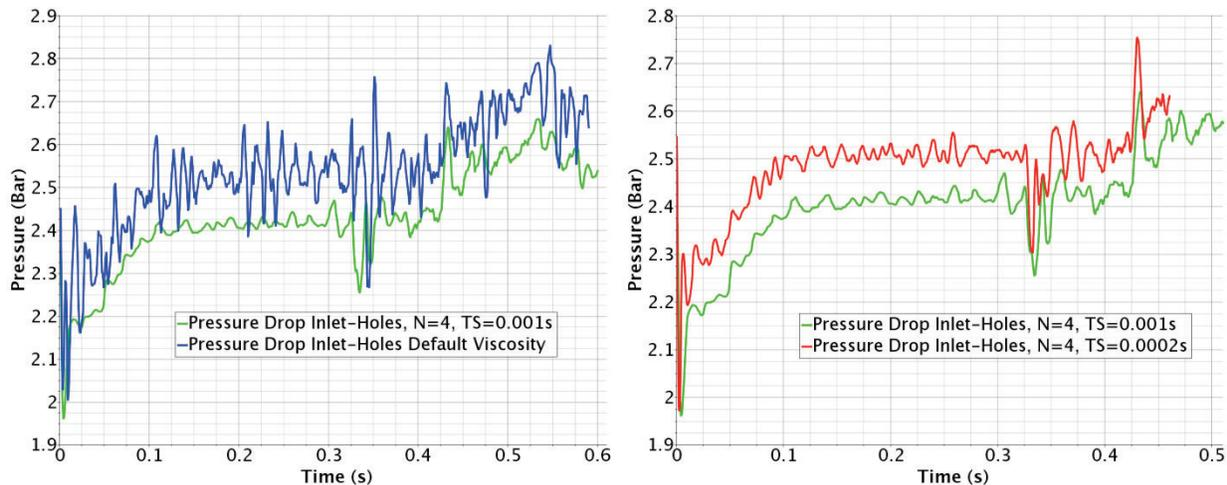
**Figure 13: Pressure drop LBE default/increased viscosity (left), different time steps (right)**
