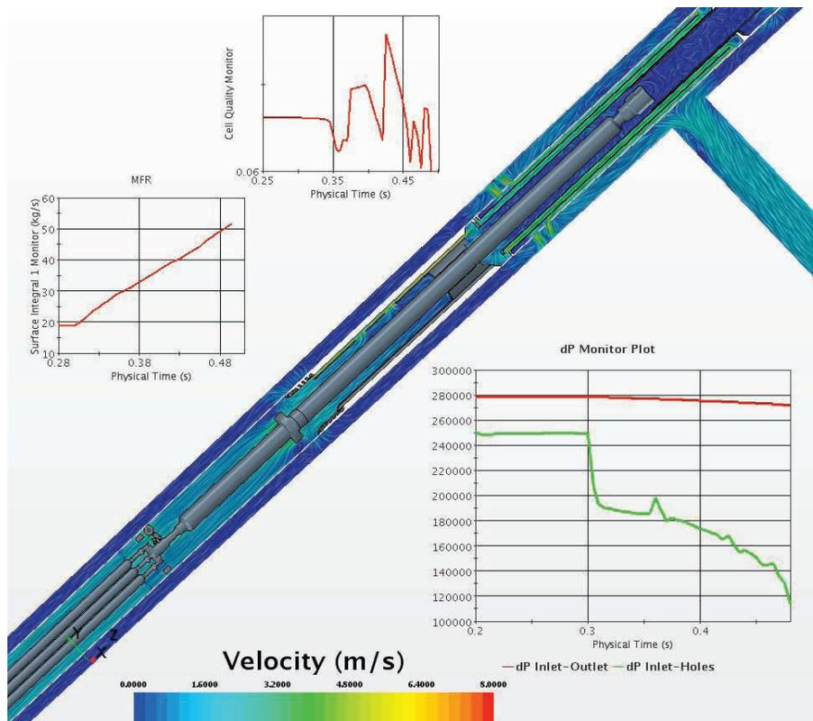
Figure 3: End of the first part of the movement, performed with morphing and re-meshing
