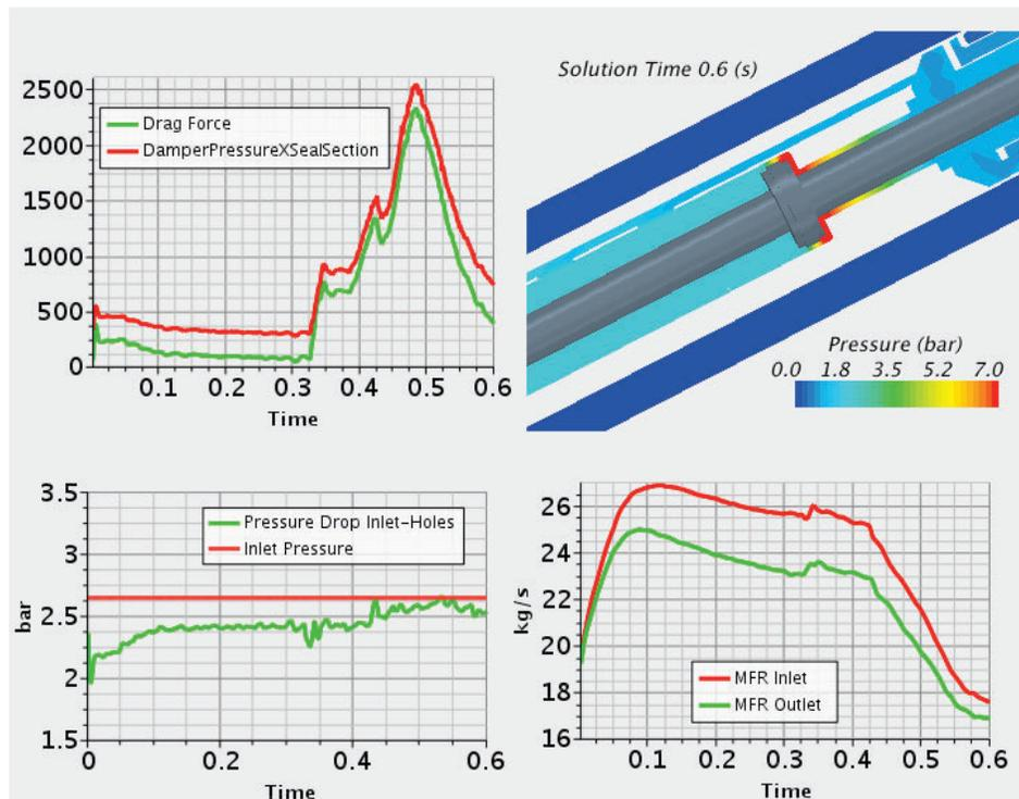
Figure 12: Drag force and pressure in the damper in full correspondence
