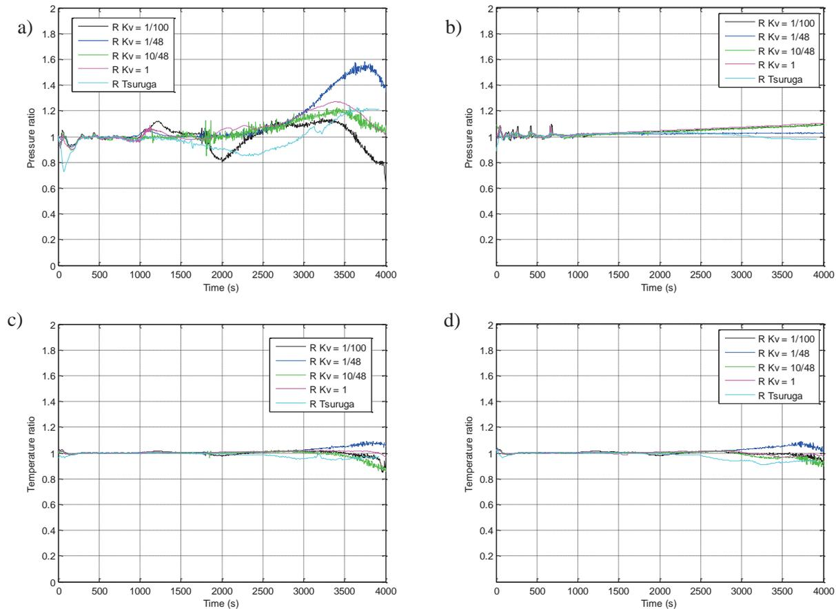
**Figure 7. For different scale models, the ratio between simulated and experimental for: a) primary pressure, b) secondary pressure, c) CET and d) PCT values.**
