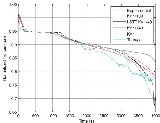
**Figure 5. CET for different scale models in comparison with experimental data.**
