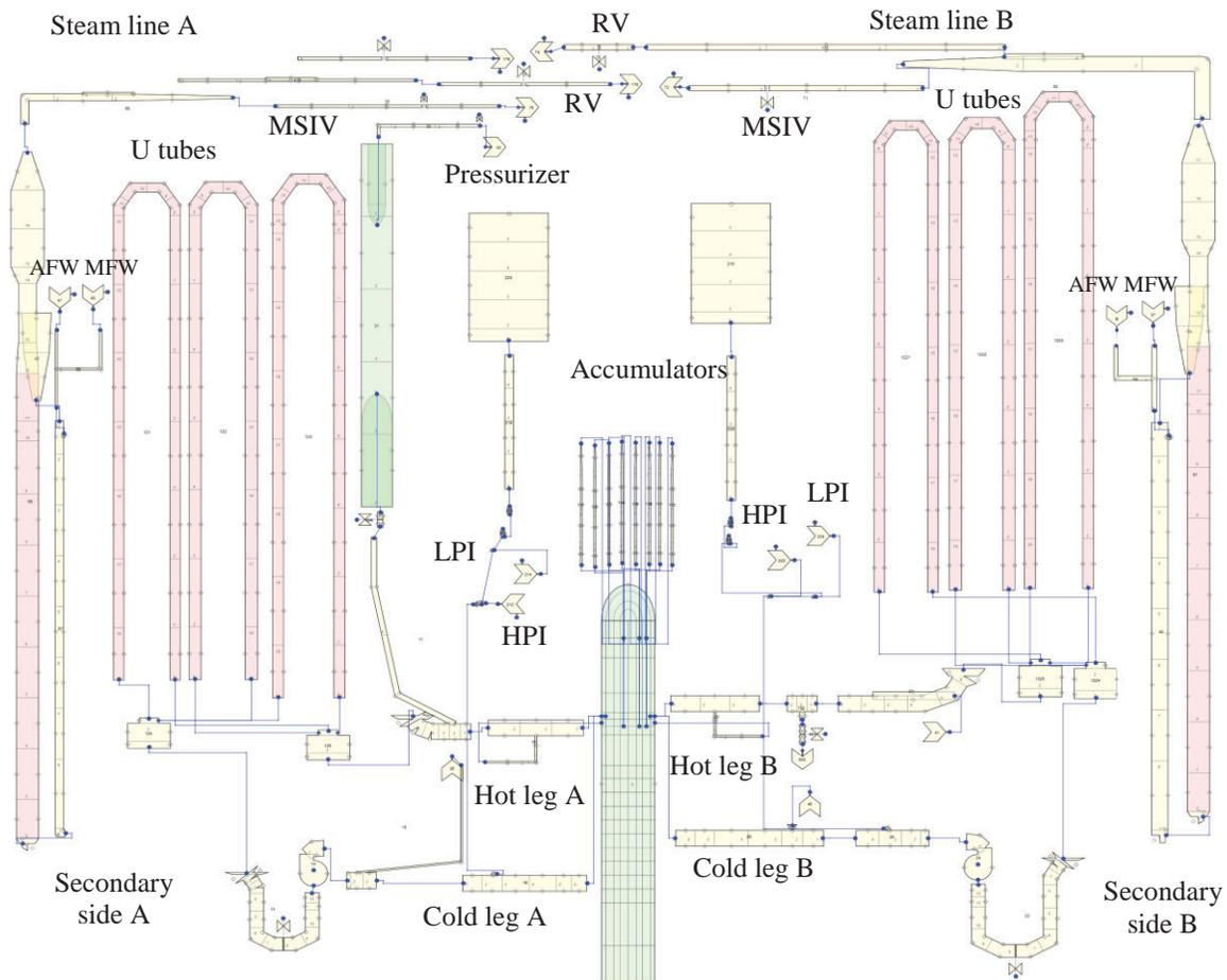
**Figure 1. Model nodalization of the LSTF TRACE5 model.**
