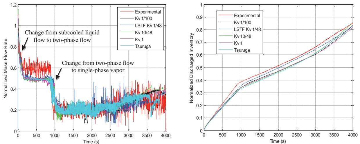
**Figure 4. a) The mass flow rate and b) the discharged inventory through the break for different scale models in comparison with experimental data.**
