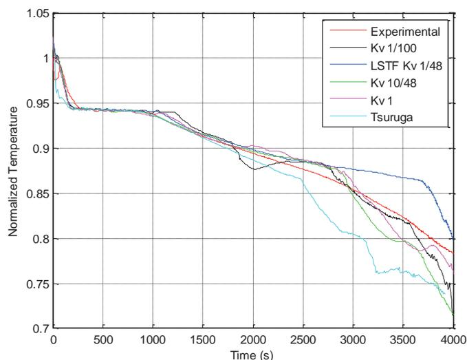
**Figure 6. PCT for different scale models in comparison with experimental data.**
