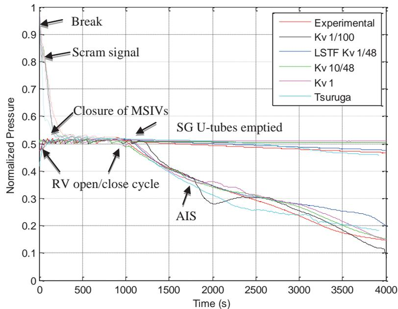
**Figure 2. The system pressures for different scale models in comparison with experimental data.**
