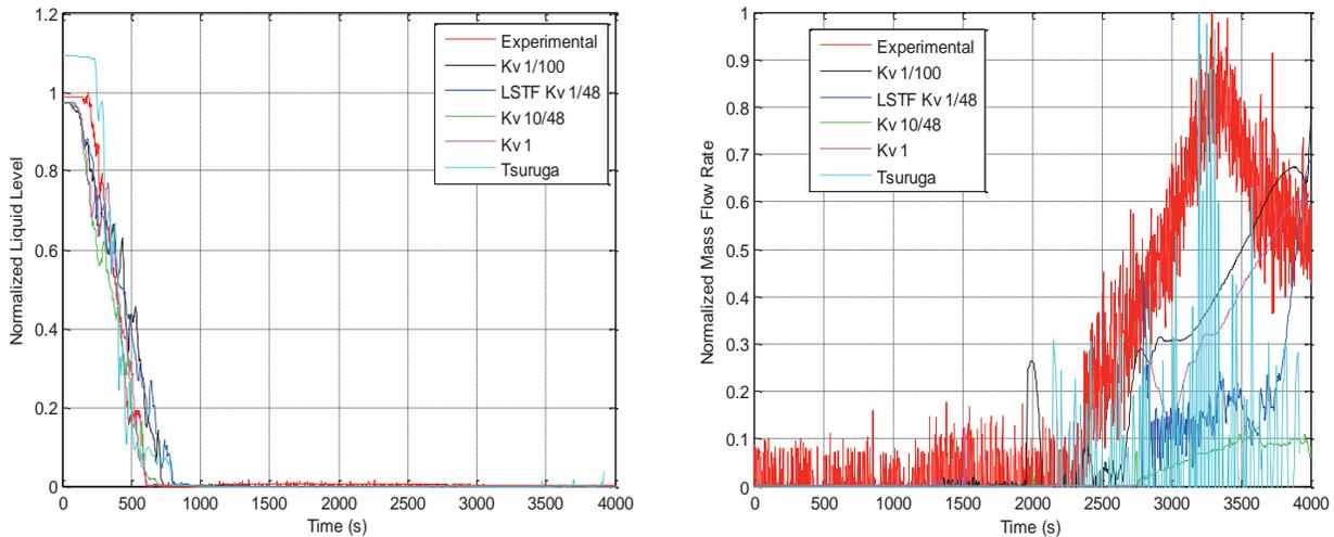
**Figure 3. a) The SG U-tubes liquid level and b) the AIS mass flow rates for different scale models in comparison with experimental data.**
