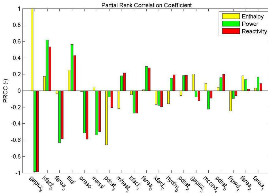
Figure 5: Maximum peak approach, PRCC for the most sensitive input parameters (PCRR > 0.16) using LHS sampling method.
