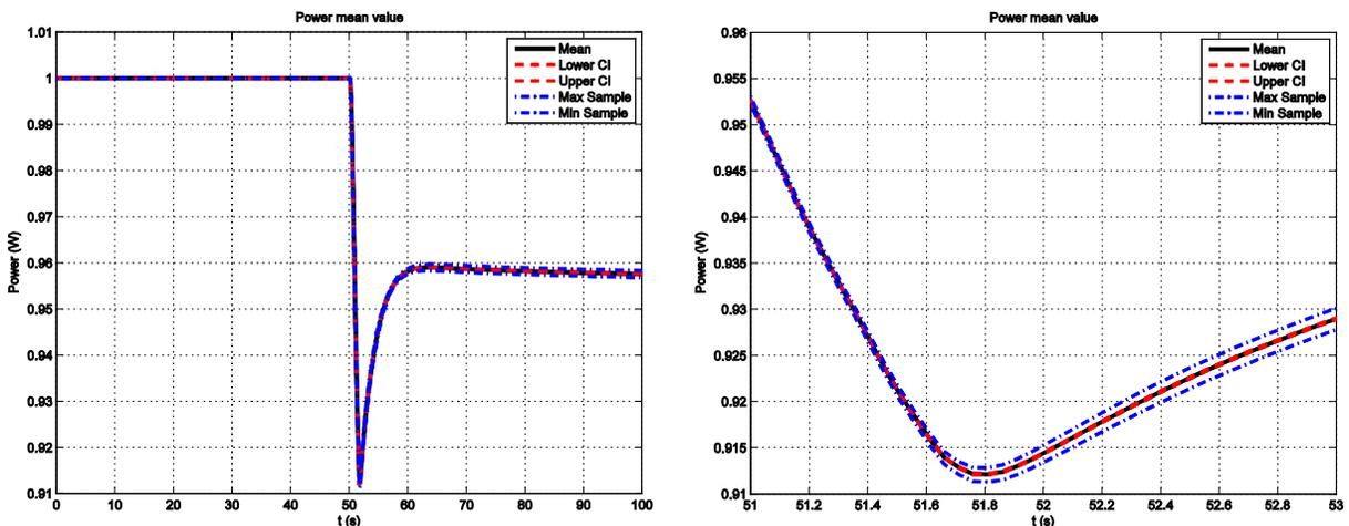
**Figure 8: Power mean (solid black line), the lower and upper 95% confidence interval (dashed red lines) and the maximum/minimum for each time step among all samples (dot-dashed blue lines). LHS sampling results. Peak zoom is shown on the right.**
