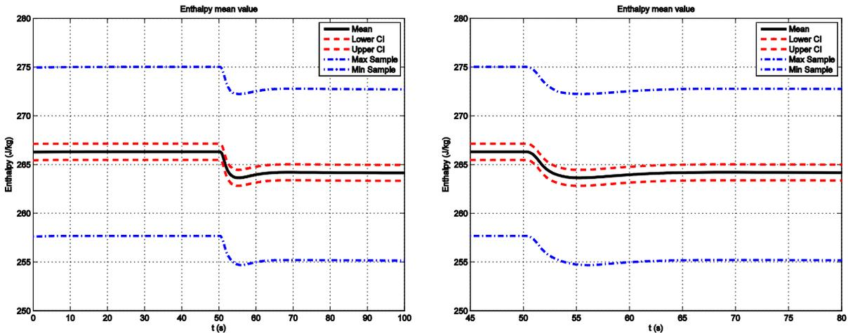
**Figure 7: Enthalpy mean (solid black line), the lower and upper 95% confidence interval (dashed red lines) and the maximum/minimum for each time step among all samples (dot-dashed blue lines). LHS sampling results. Peak zoom is shown on the right.**
