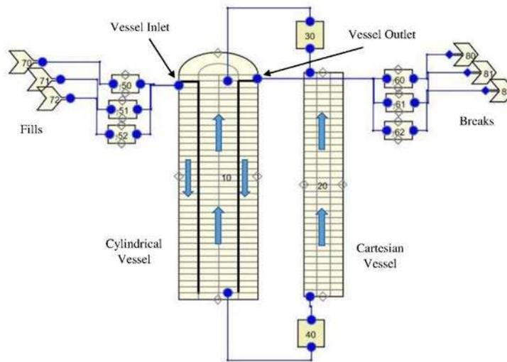
**Figure 3: Simplified TRACE model for PWR 3D core representation by means of a cartesian vessel (fuel assemblies) and a cylindrical vessel (inner radial cell bypass and outer cell downcomer), sketch using SNAP tool.**
