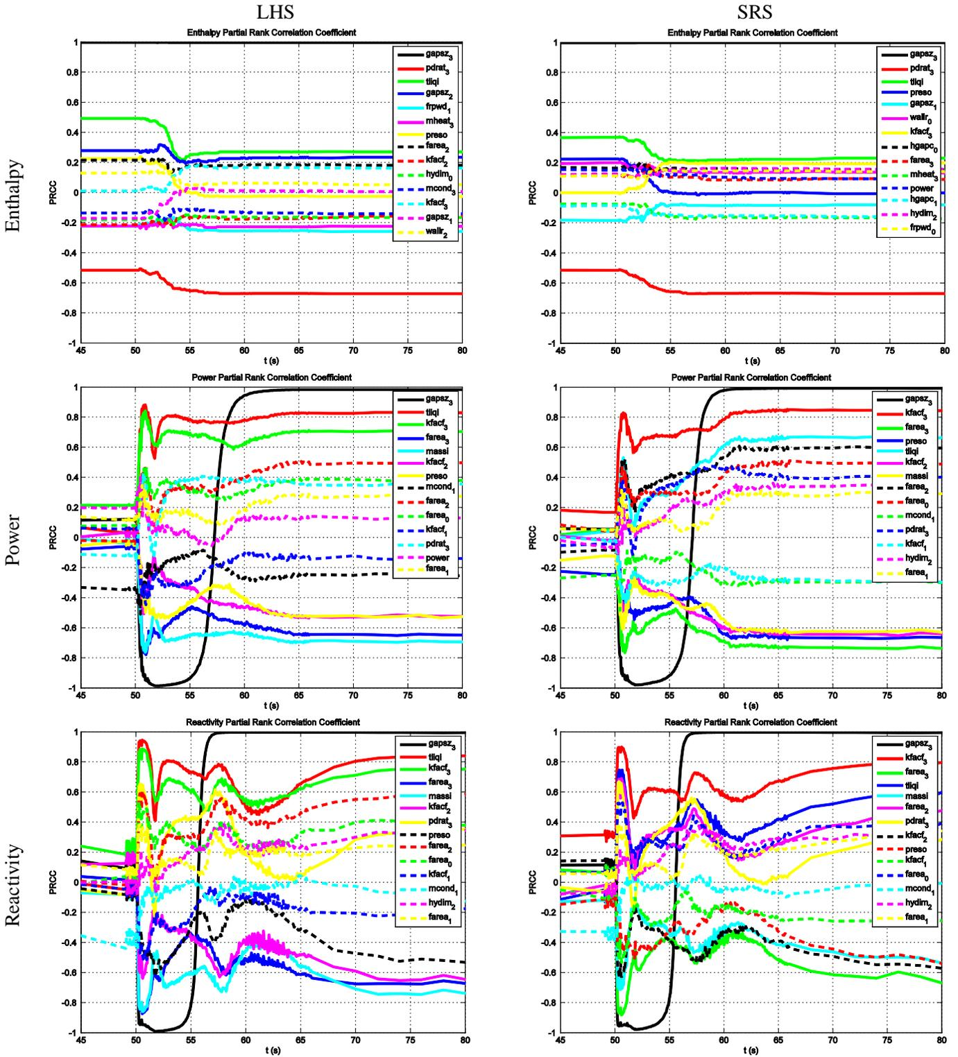
Figure 11: Index dependent approach, PRCC for the most sensitive input parameters and the output parameters (enthalpy, power & reactivity). Left column contain LHS sampling method results, whereas right column shows the results for the SRS sampling method.
