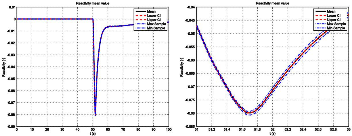
**Figure 9: Reactivity mean (solid black line), the lower and upper 95% confidence interval (dashed red lines) and the maximum/minimum for each time step among all samples (dot-dashed blue lines). LHS sampling results. Peak zoom is shown on the right.**
