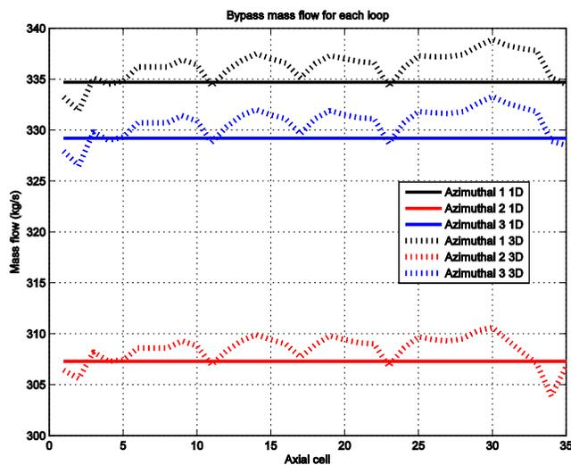
**Figure 4: Bypass flow for three different azimuthal sectors comparing TRACE 3D model (dotted lines) and RELAP 1D equivalent model (stright lines), flow as function of axial cells in axial direction.**
