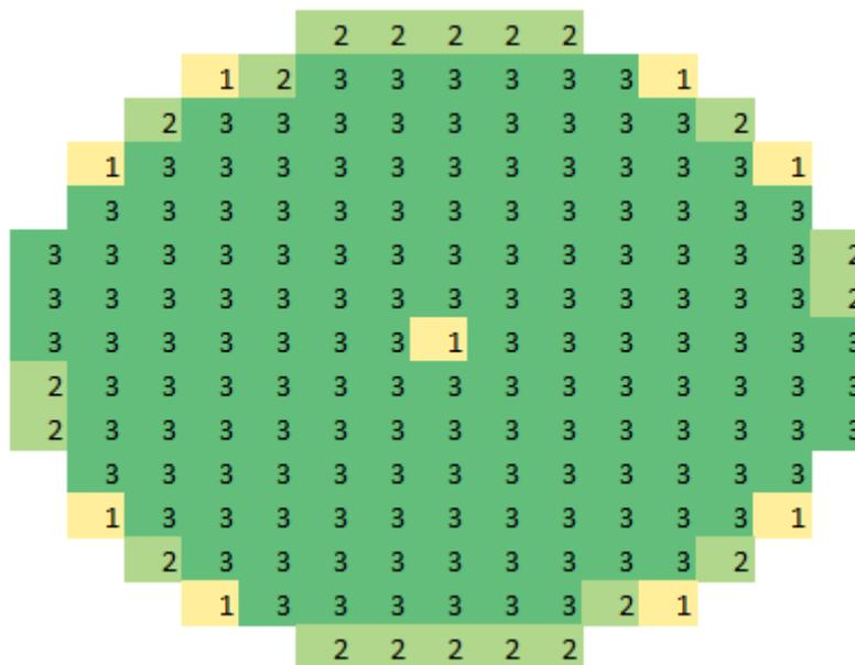
**Figure 12: Fuel type radial mapping.**
