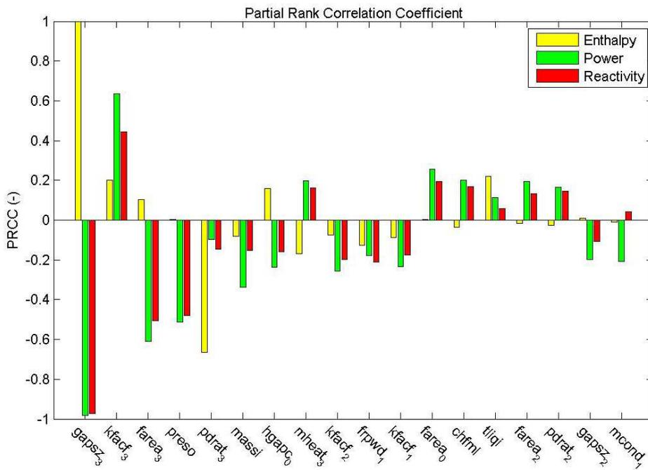
Figure 6: Maximum peak approach, PRCC for the most sensitive input parameters (PCRR > 0.16) using SRS sampling method.
