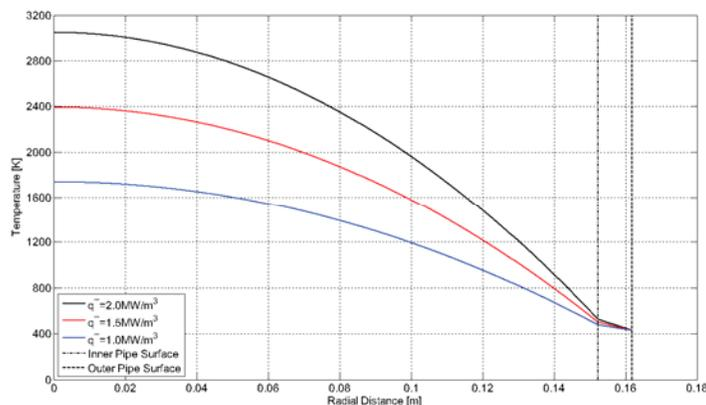
**Figure 5: Temperature profile of corium in a penetration**
