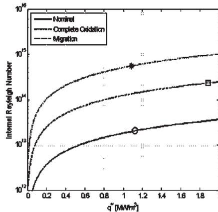
**Figure 3: Variation of Rayleigh number with volumetric heat generation rate**
