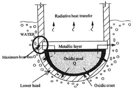
Figure 1: Two-layer corium pool configuration [18]
