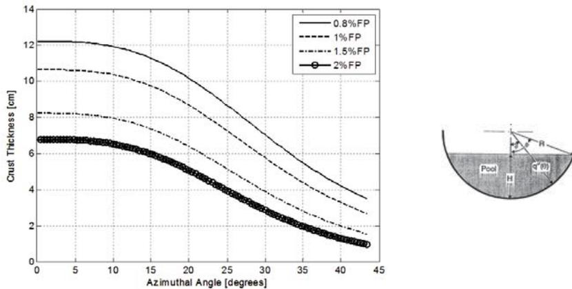
**Figure 4: Variation of lower crust thickness with azimuthal angle**
