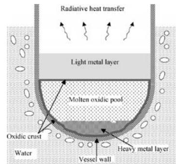
Figure 2: Three-layer corium pool configuration [17]
