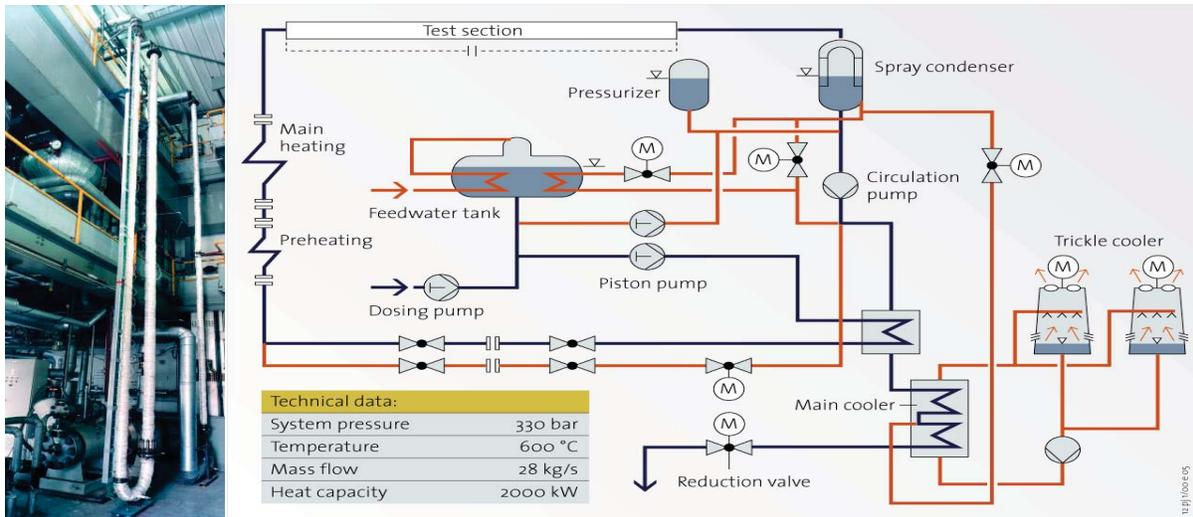
Figure . 1: BENSON Test rig scheme and a photo with integrated test tube
