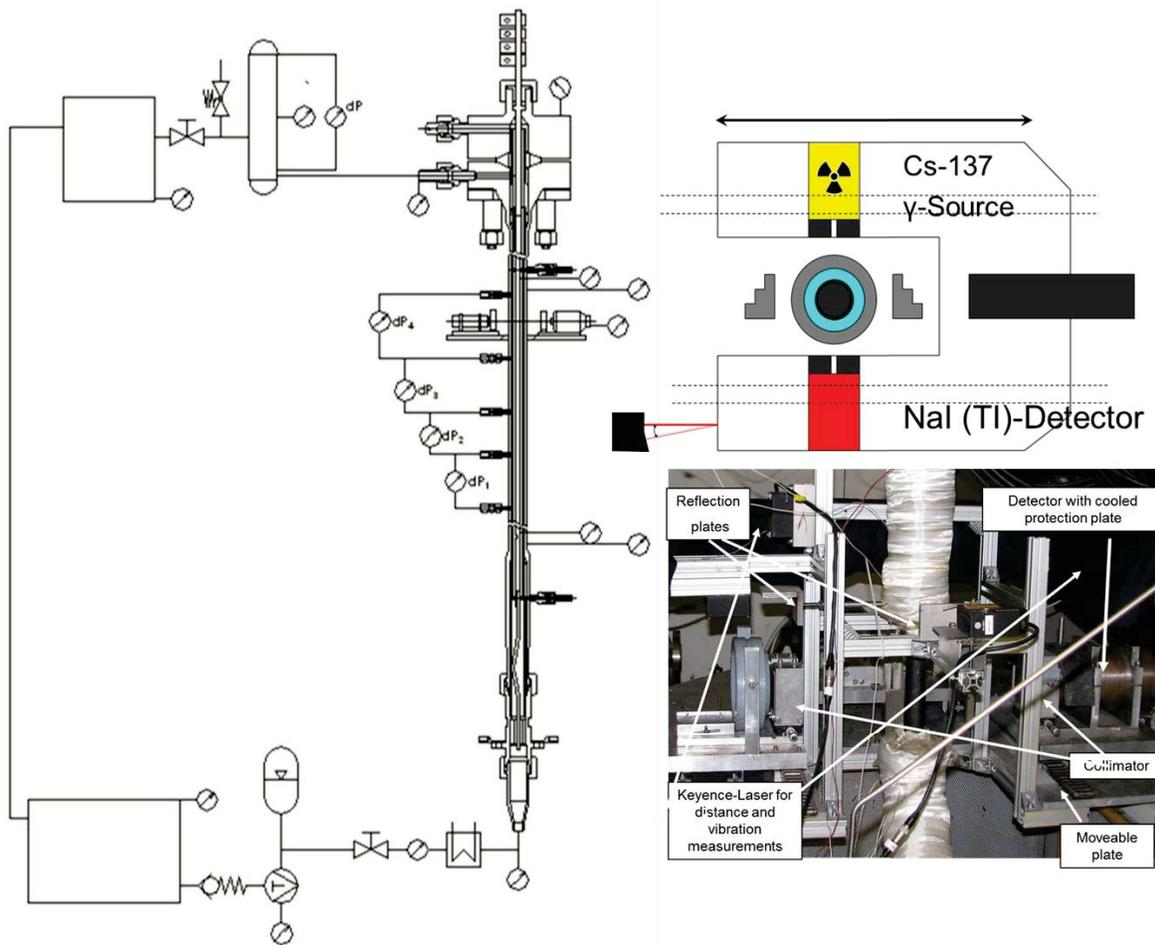
**Figure 5:** left: scheme of the calibration loop – right top: arrangement of the gamma densitometer – right bottom: photo of an arrangement of a gamma densitometer
