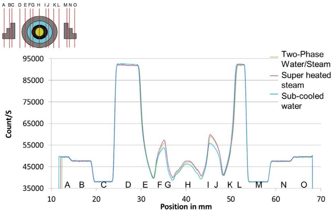
**Figure 6:** Beam intensity along the test channel and the related calibration blocks
