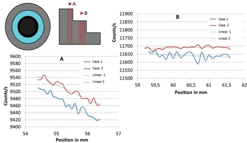
**Figure 8:** Beam intensity measurements along calibration blocks
