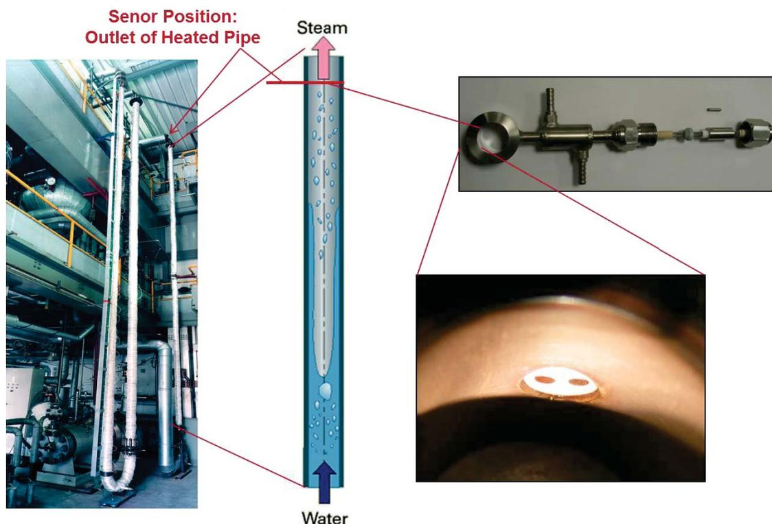
**Figure 12:** Arrangement of a high pressure impedance probe
