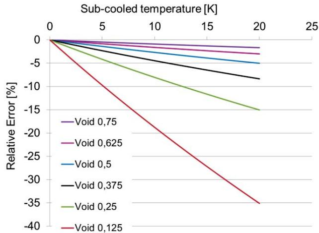
**Figure 9:** Error without considering the sub-cooling in the evaluation process at 70 bar
