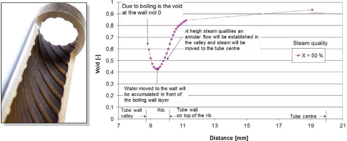
Figure 2: Void fraction distribution in a rifled tube as shown on the left picture
