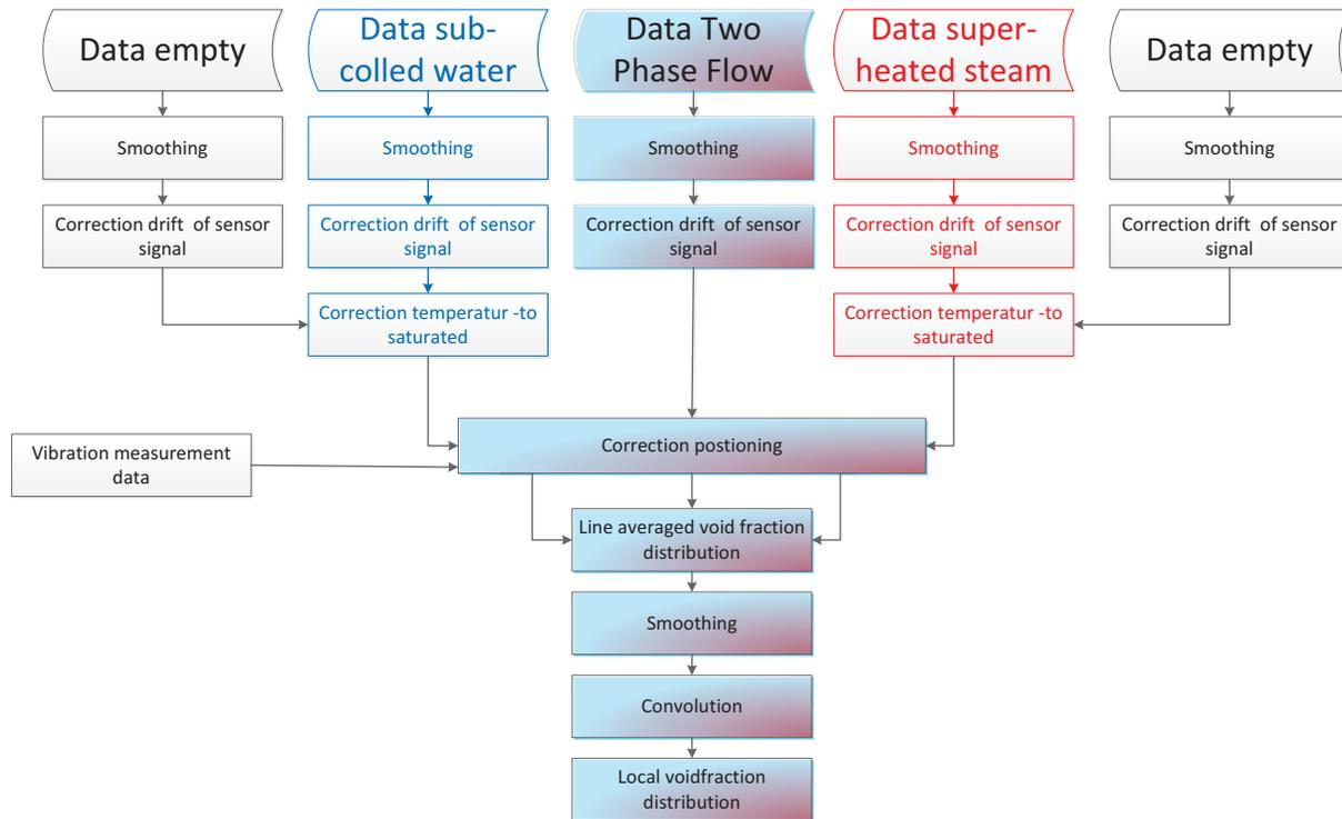
**Figure 7:** Evaluation process to determine the local void fraction distribution
