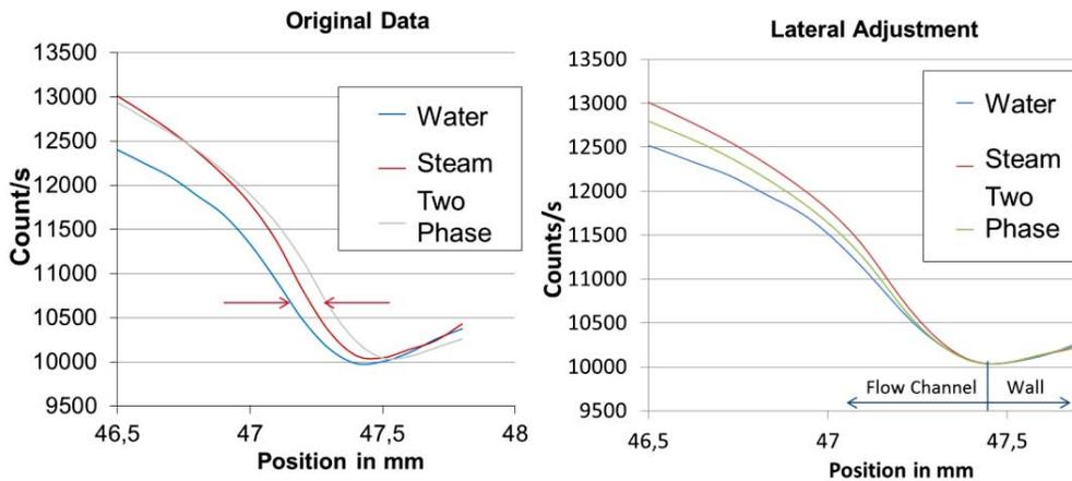
**Figure 10:** Adjustment of the water, steam and two phase flow profiles to inner wall position
