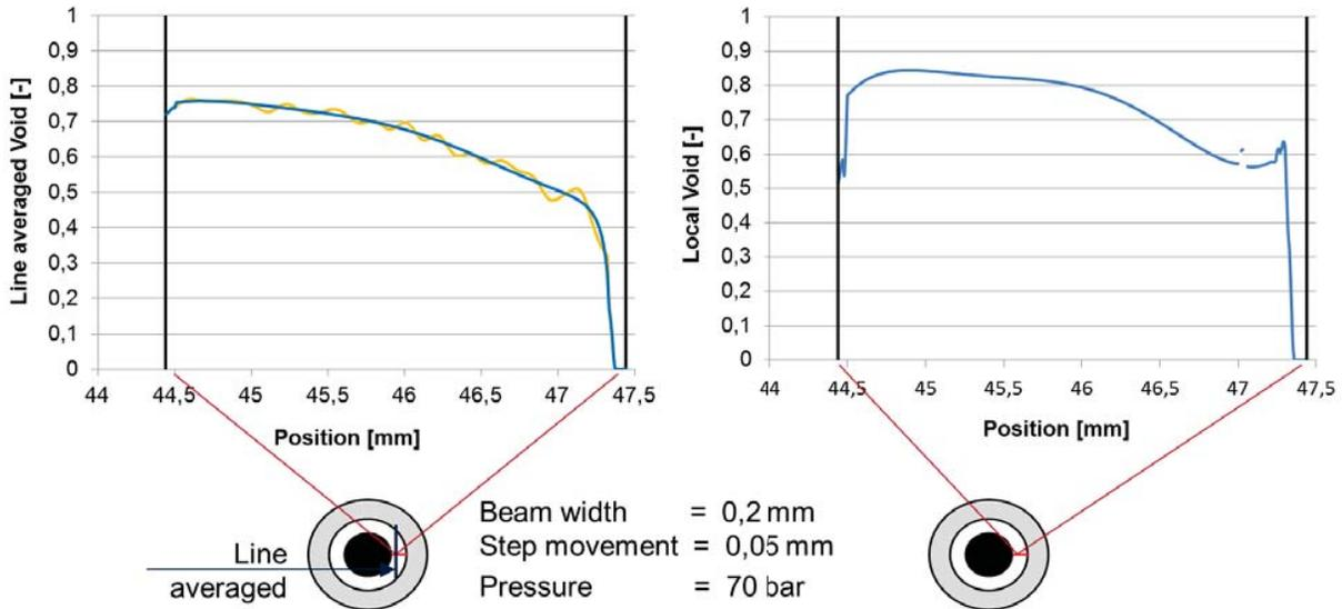
**Figure 11:** Local and line averaged void fraction distribution in a water column with steam supply
