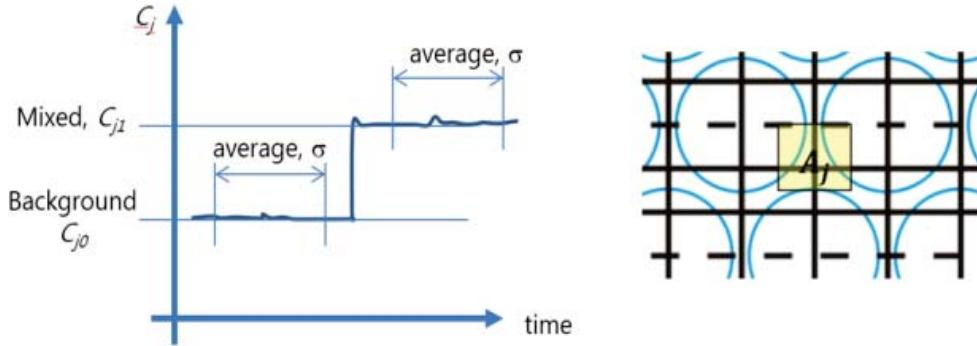
**Figure 4. Test procedure and definition of area factor ( $A_j$ ).**
