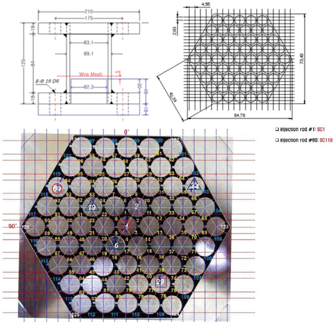
**Figure 3. Design of our wire mesh sensor and matching with our 61-pin assembly.**
