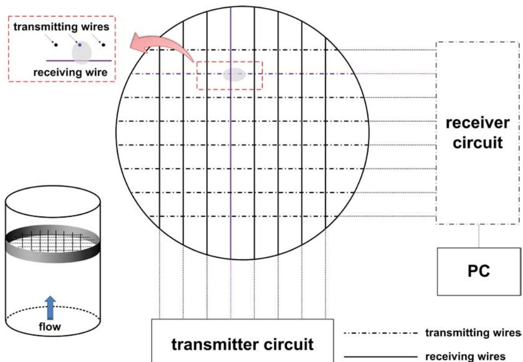
**Figure 2. Principle of a wire-mesh sensor.**
