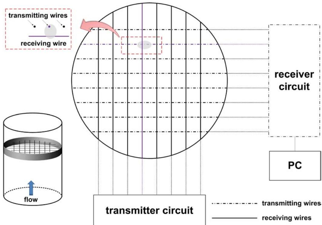
**Figure 2. Principle of a wire-mesh sensor.**
