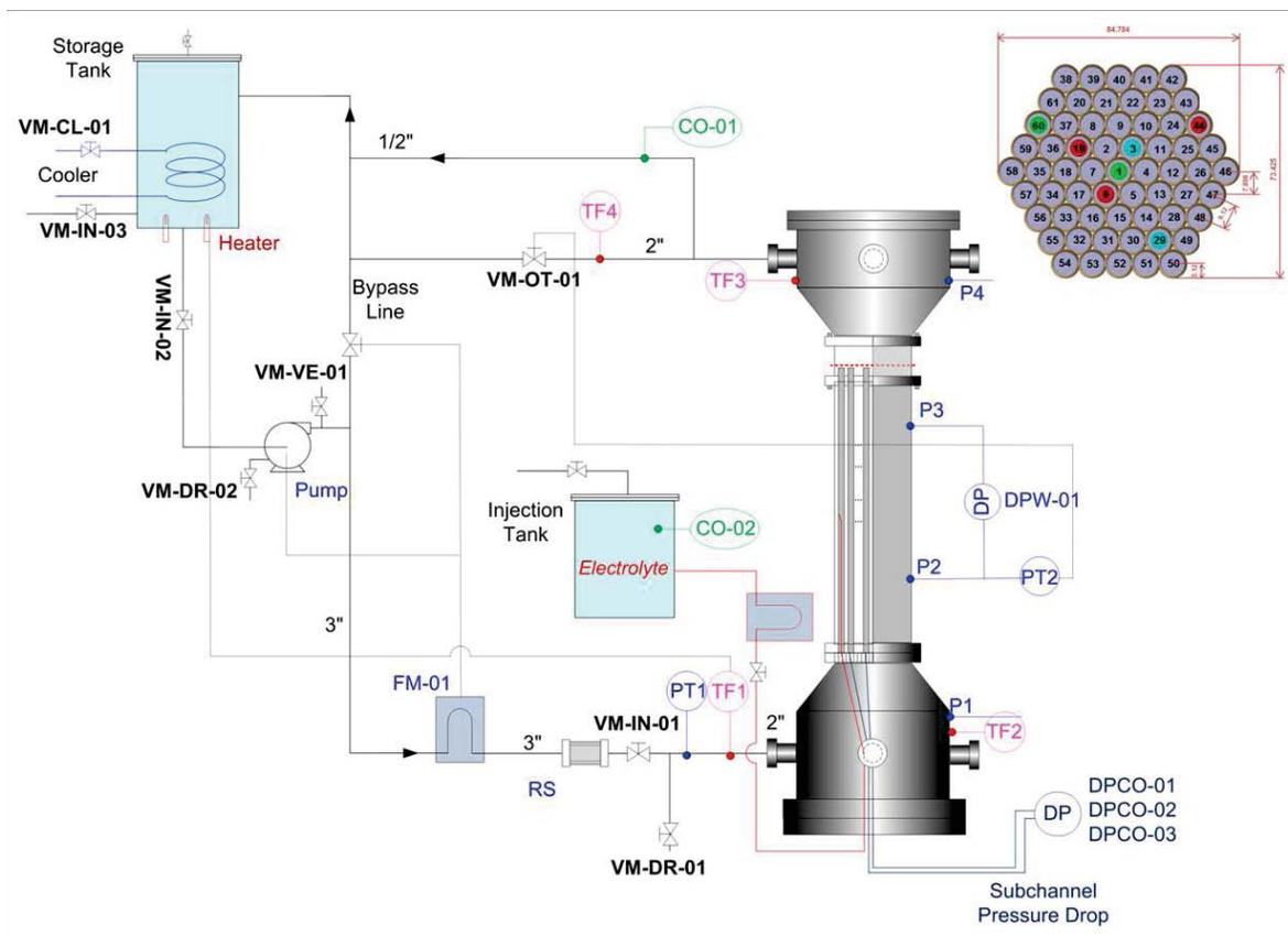
**Figure 1. Schematic of the test loop for measurements of flow mixing.**
