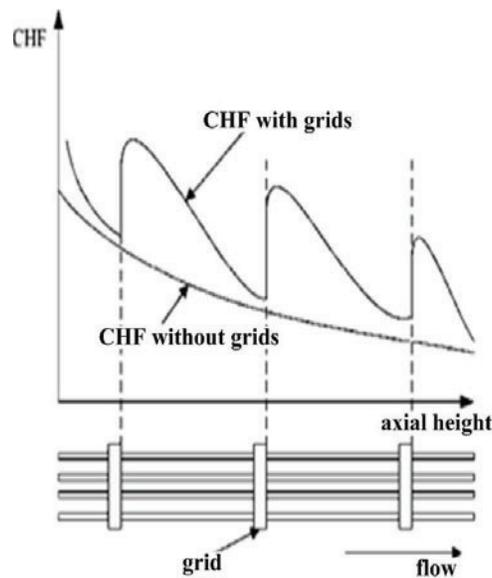
**Figure 3. CHF distribution of fuel assembly with mixing vane**
