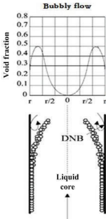
**Figure 2. Fluid thermohydraulic Condition in a tube on DNB**
