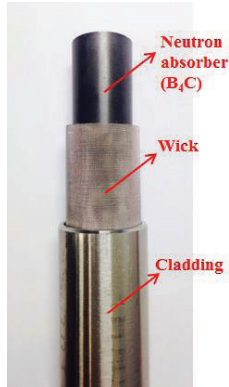
Figure 2. Composition of hybrid control rod.
