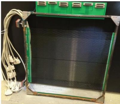
(b) Tank wire-mesh sensor.
