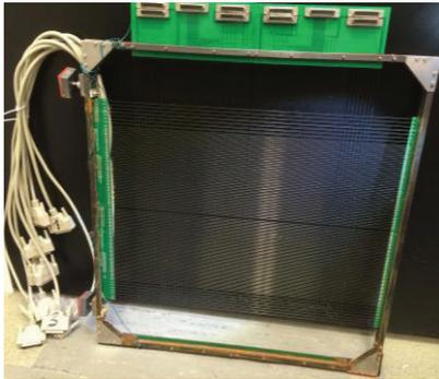
(b) Tank wire-mesh sensor.
