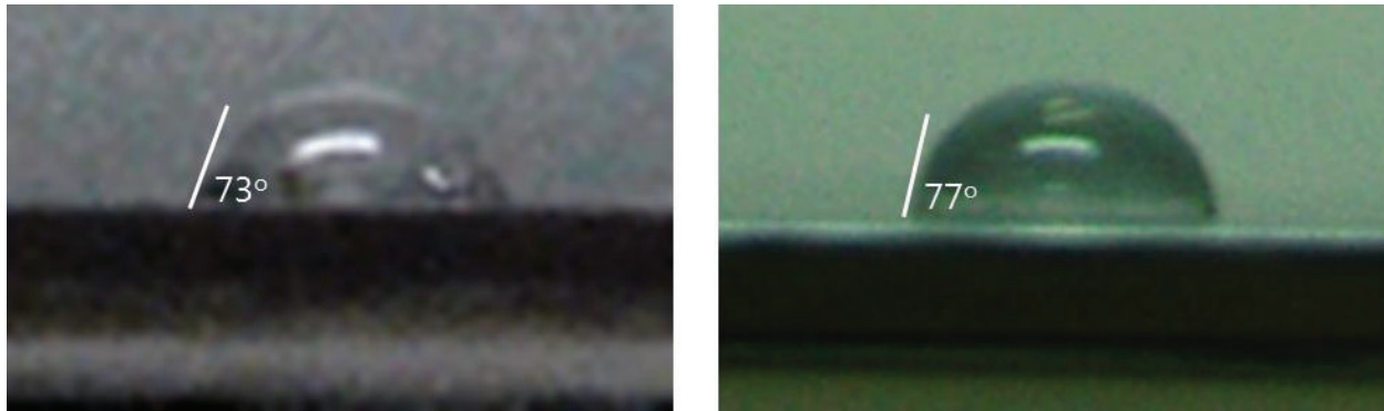
Figure 9. Contact angle measurements of two surfaces before experiments (Left: SUS 304, Right: SA 508).
