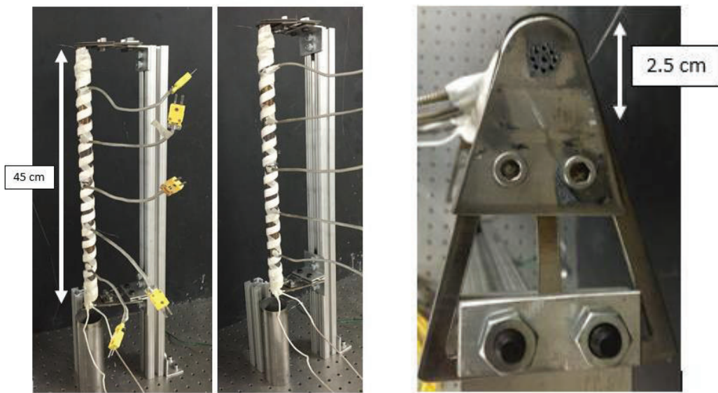
Figure 1. Optical fiber high temperature testing oven. Shown without thermal insulation applied.
