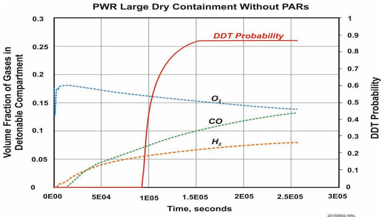
Figure 5: DDT Probability of Severe Accident Sequence in Example PWR without PARs
