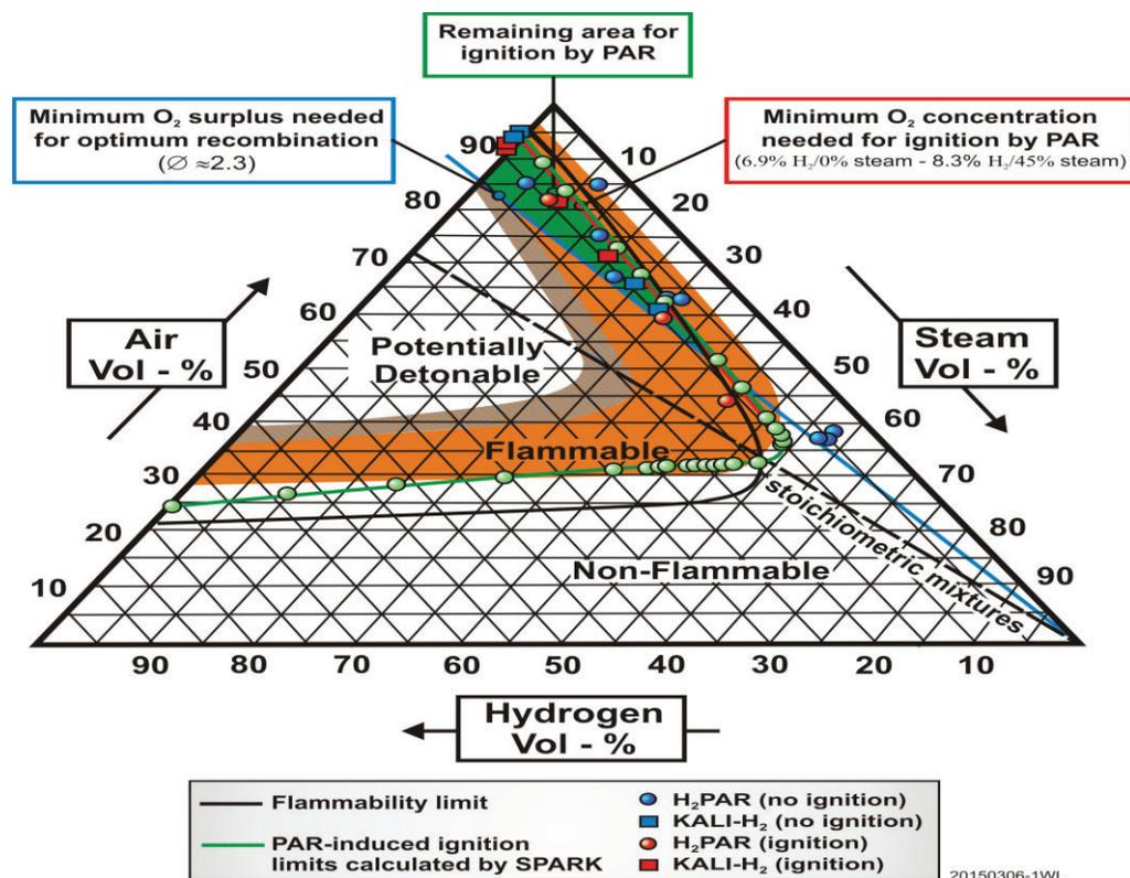
Figure 2: Flammability Limits [8] and PAR-induced Ignition Limits [9].
