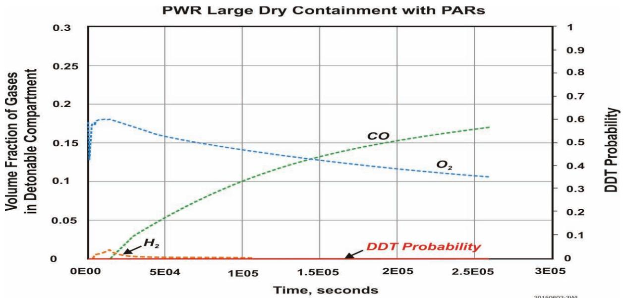
Figure 6: DDT Probability of Severe Accident Sequence in Example PWR with PARs
