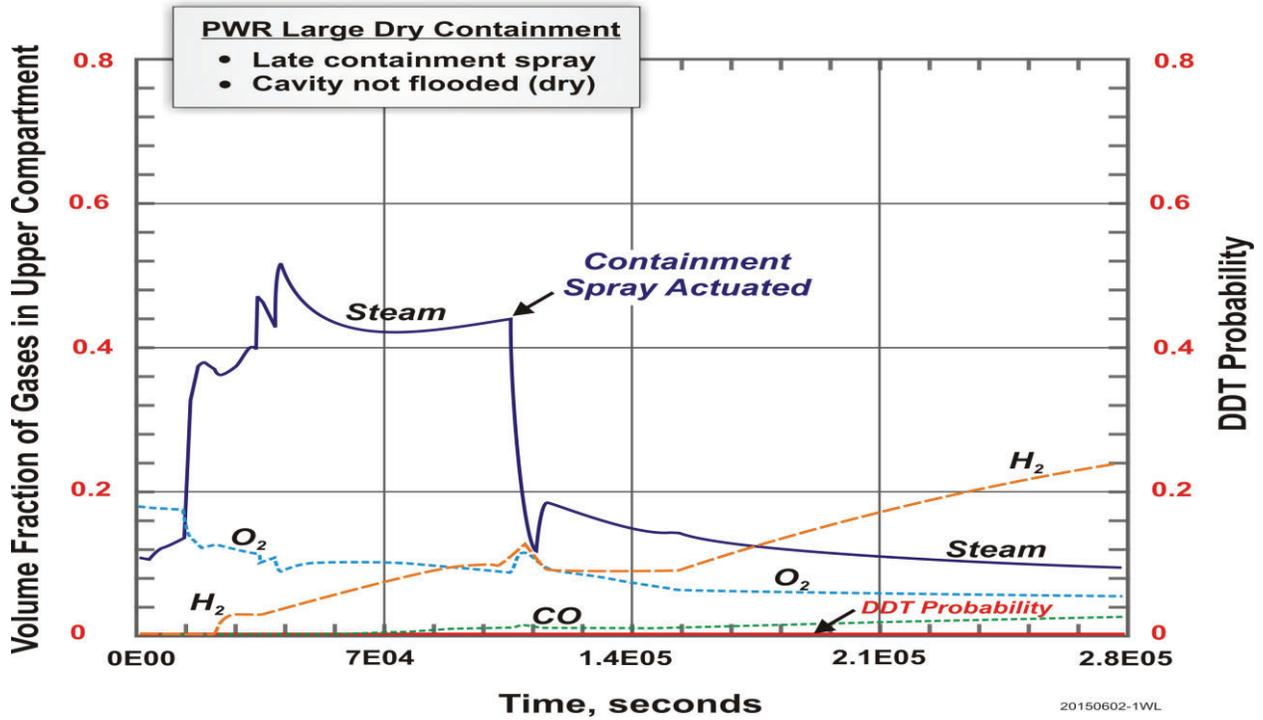
Figure 4: DDT Probability of Severe Accident Sequence in Example PWR with Late Containment Spray actuated but Cavity remained Dry
