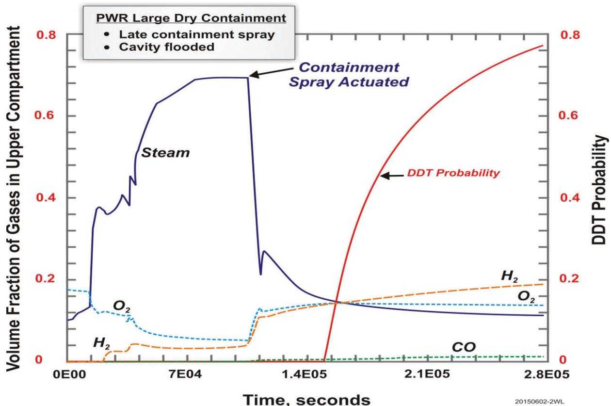
Figure 3: DDT Probability of Severe Accident Sequence in Example PWR with Flooded Cavity due to Late Containment Spray Actuation
