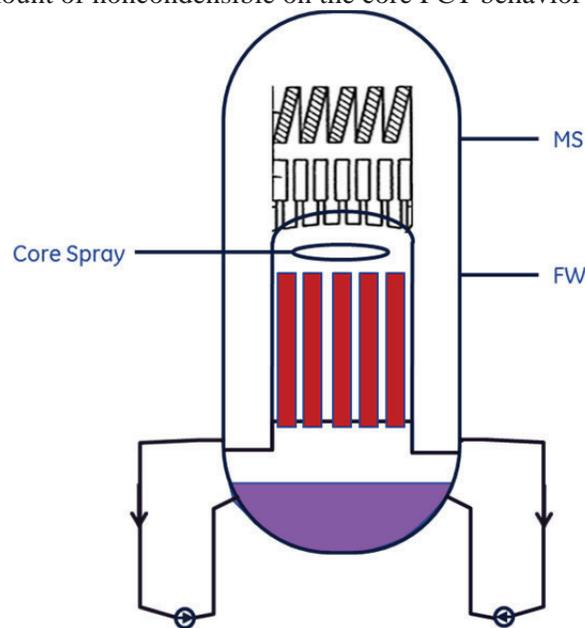
**Figure 1. Schematic of a Typical BWR/2 Core and Recirculation System.**
