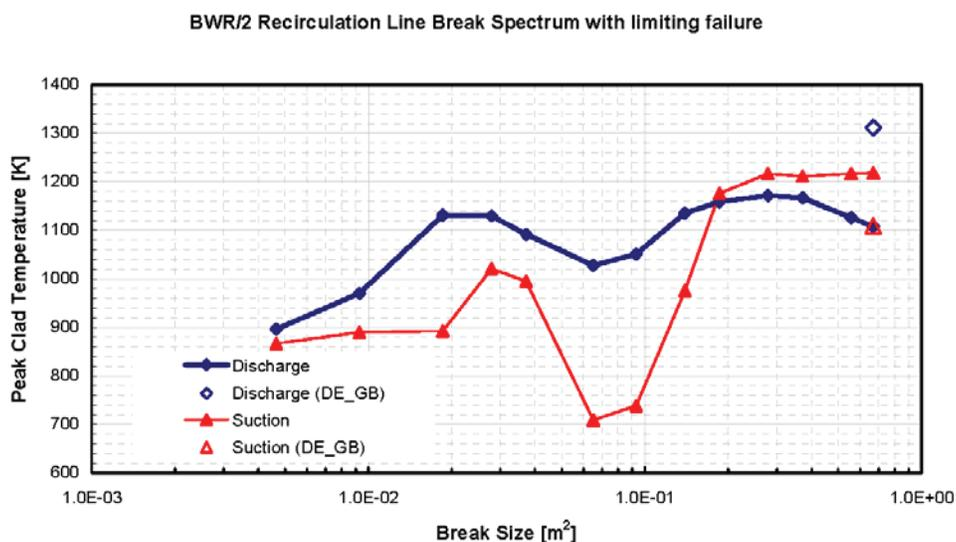
Figure 3. Break Spectrum for BWR/2 Discharge and Suction Side Breaks with Air Break Boundary Conditions.
