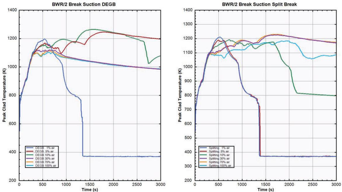
Figure 10. PCTs for different Break boundary conditions for SUCT.
