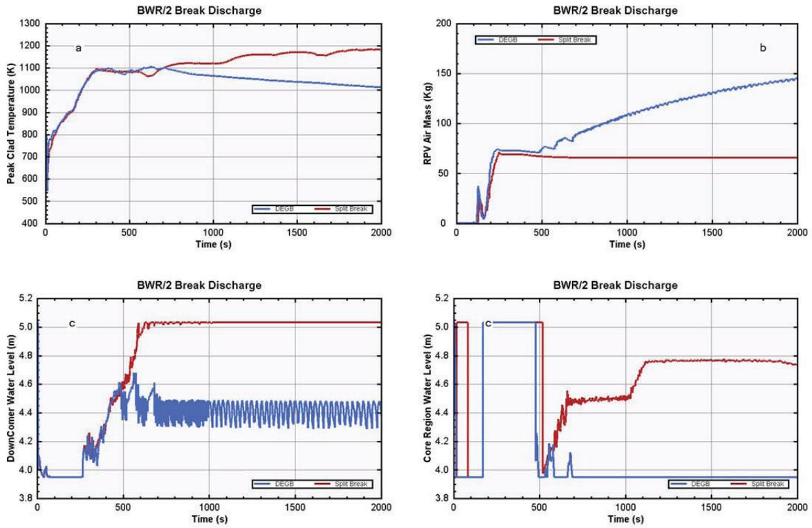
Figure 7. Comparisons for BWR/2 Suction DE GB and the same break area Split break.
