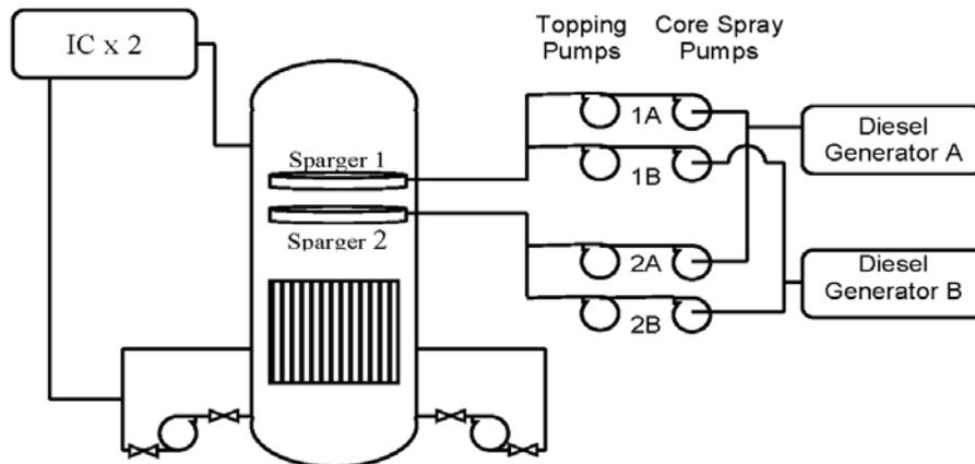
Figure 2. A Typical BWR/2 ECCS Configuration.
