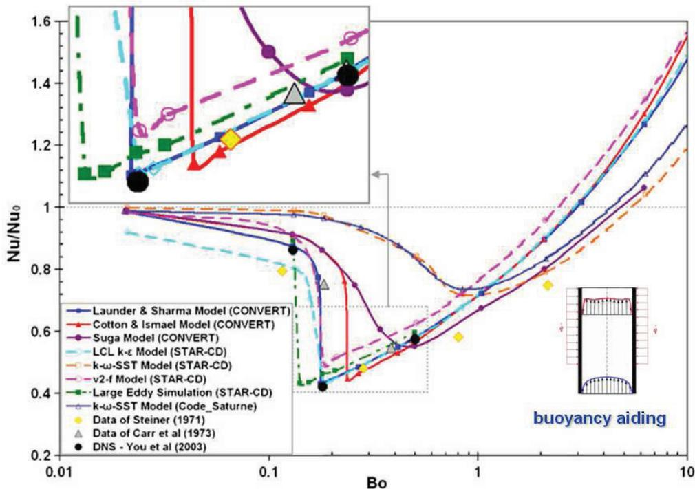
Figure 4. Ratio of mixed-to-forced convection Nusselt number as a function of the buoyancy parameter by several RANS models, LES and DNS for an ascending mixed convection flow [33].
