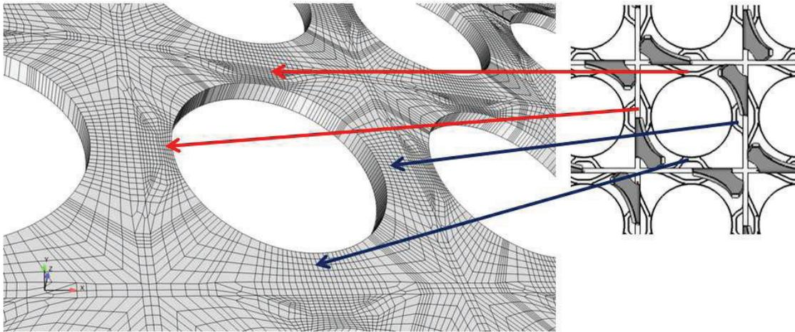
Figure 2. Mesh cut downstream a grid with mixing vanes.
