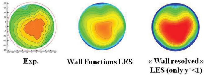
Figure 7. Mean stream-wise velocity component downstream a T-junction.
