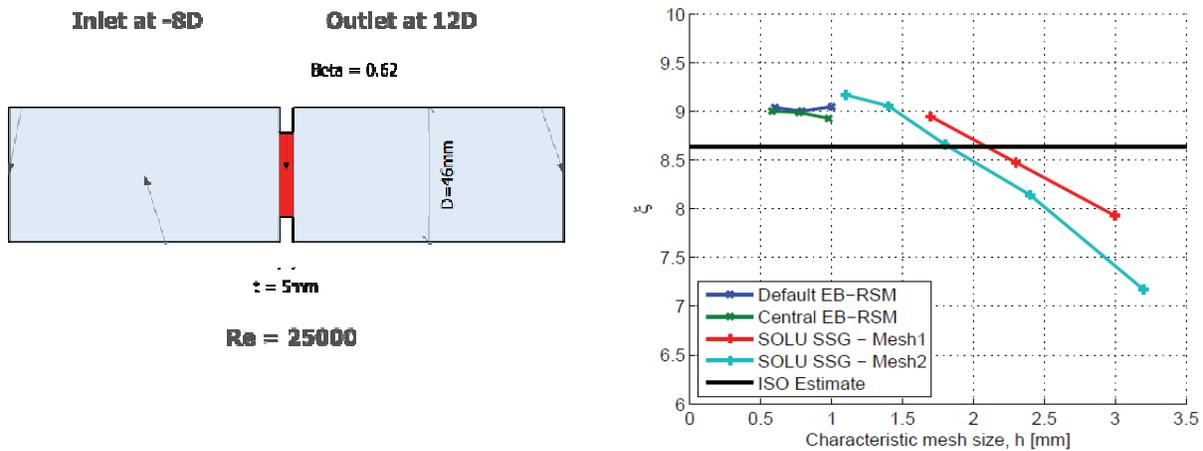
Figure 3. Left: Computational domain for the square edged circular orifice plate, Right: Pressure loss across the orifice versus mesh refinement.
