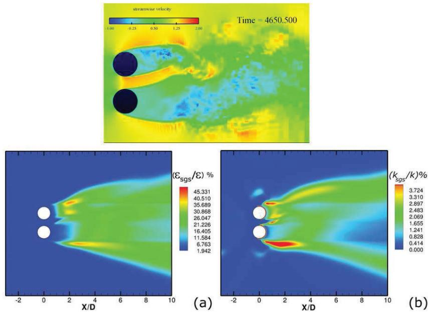
Figure 8. The flow around two side-by-side cylinders at subcritical Reynolds numbers – estimates of the sub-grid scale dissipation rate and sub-grid scale kinetic energy.
