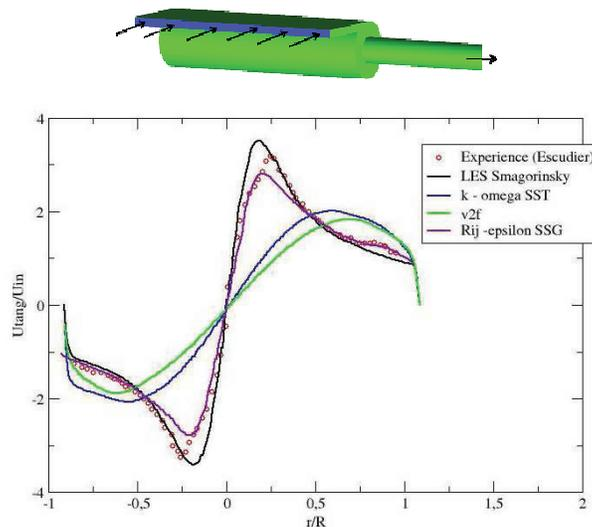
**Figure 1. Top: Confined Vortex Tube Geometry, bottom: Tangential velocity in the large pipe.**
