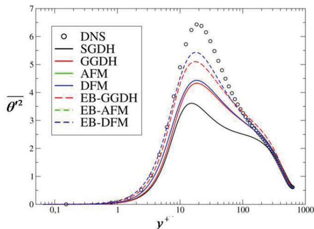
Figure 5. Temperature variance, forced convection, channel flow,  $Re_\tau=640$ ,  $Pr=0.71$ , comparisons to DNS data from [37].
