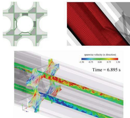
**Figure 9. Flow through a mixing grid at  $Re=40000$ . Top left: cut of the computational domain (2x2 periodic bundle), top right: hexahedral mesh (8 million cells), bottom: snapshot of the instantaneous cross-stream velocity.**
