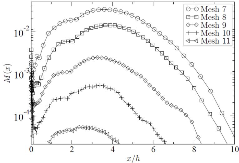
**Figure 6. Maximum resolved energy/total energy ratio as a function of the stream-wise location for successive mesh refinements. Mesh 12, finest, gives a steady solution. Image taken from [42].**
