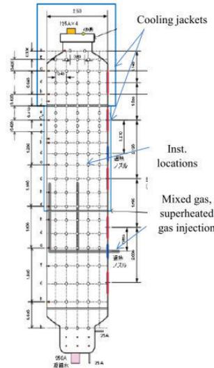
Figure 3. CIGMA Test Facility at JAEA.
