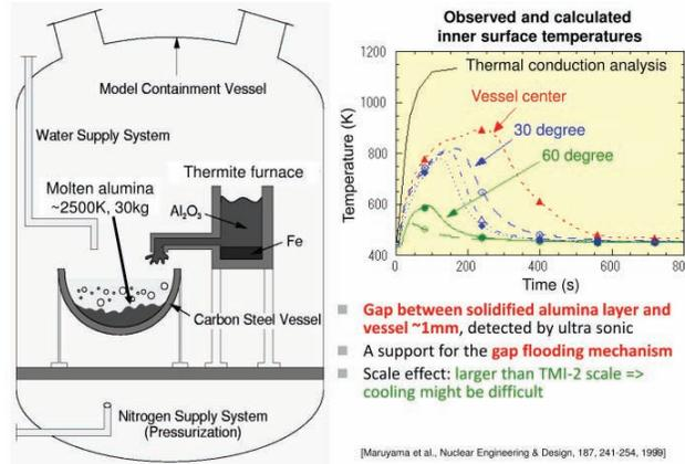
**Figure 1. In-Vessel Molten Core Coolability Experiment [15].**
