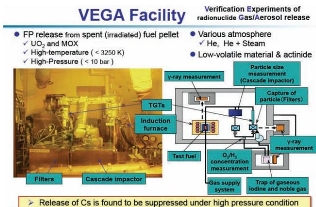
Figure 2. VEGA Experiment on FP Release from Irradiated Fuel [27].
