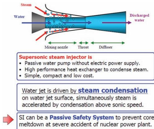
**Figure 6. Concept of Supersonic Steam Injector [43].**
